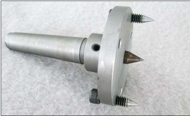
This drive center excels at holding green wood. The adjustable spikes are helpful for aligning grain and rims in natural edge bowls.
