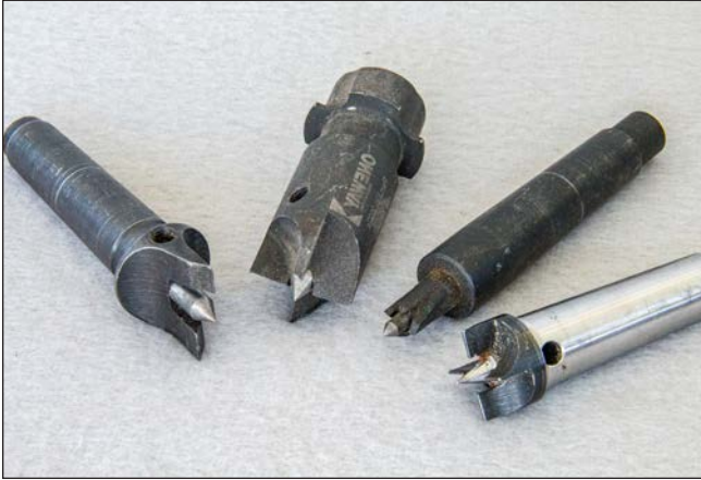
Two-spur (left) and four-spur drive centers.
