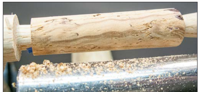
The fit of a friction drive can be fine-tuned with tape. With the hole drilled first, the outside turning is always concentric to the hole.
