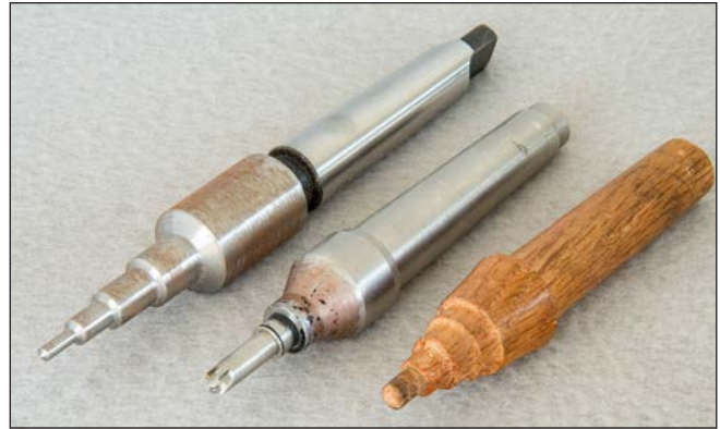
Closed end and friction drives for spindle turnings can be store-bought or shopmade.
