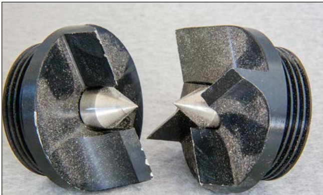
These drive centers mount quickly in chuck jaws, providing greater support for the drives than Morse taper drives.
