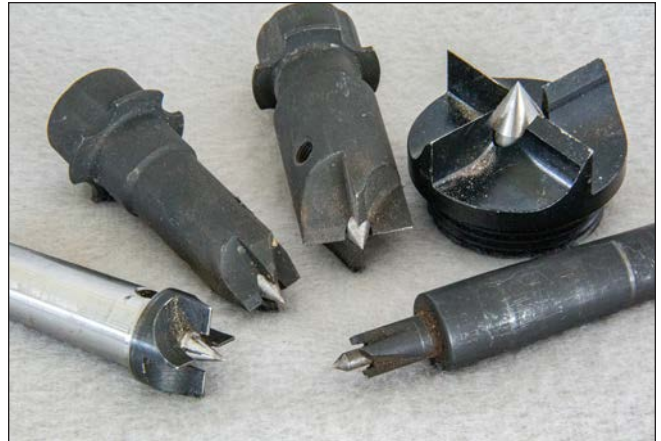
An assortment of four spur drives. Whether taper or chuck mounted, all feature adjustable center points.
