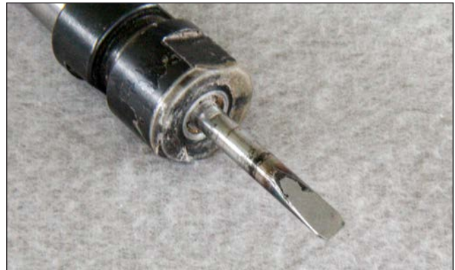
A friction drive for small-scale work. A hole bored in the end of the spindle captures the drive spur.
