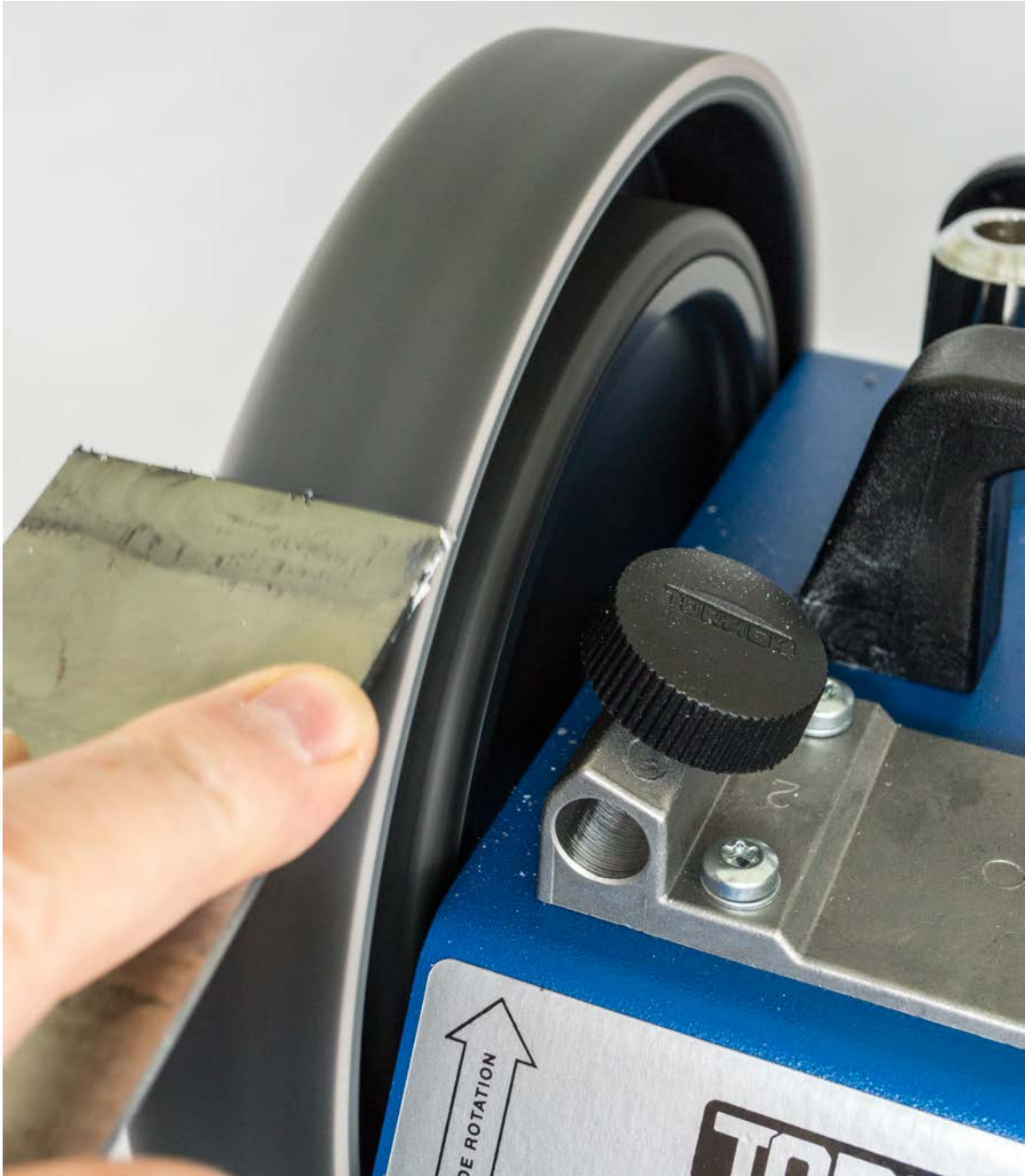
The attached leather strop and honing compound can be used immediately after sharpening without even removing the tool from the jig. It runs at the same slow rpm as the stone.
