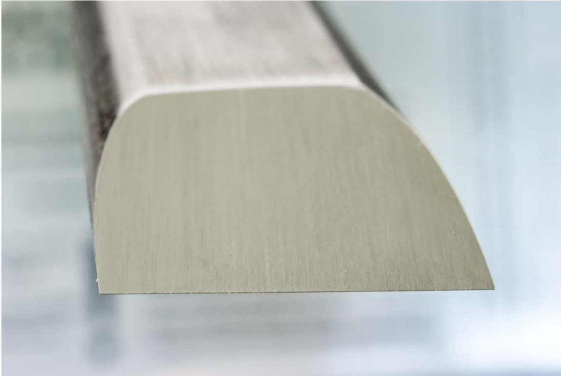
A quick look at the skew chisel after sharpening on the Tormek T-7.
