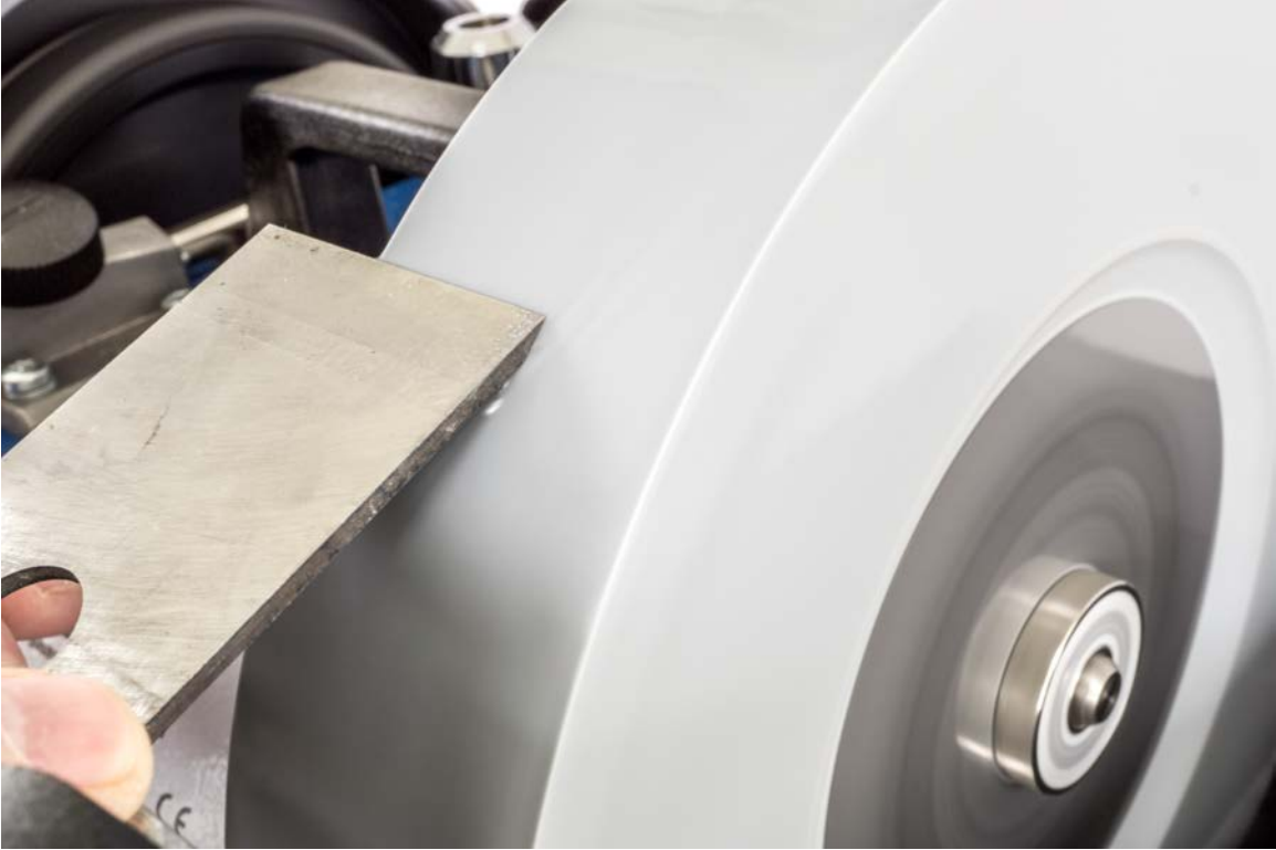
In use, the 10 inch wheel with its shallow hollow grind is a joy to use. Whether graded as coarse for additional stock removal or fine for a finer edge, the process is simple.
