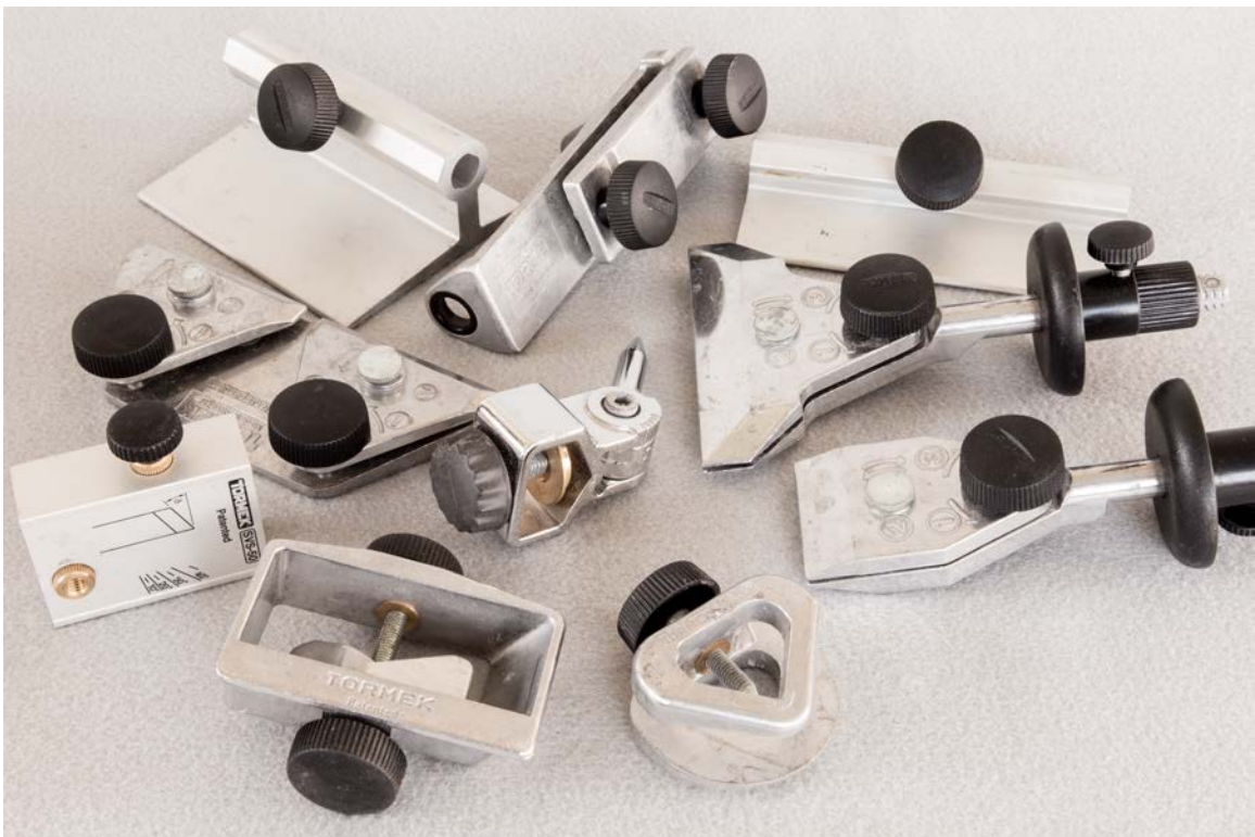
Just a few of the jigs that I've added to my system over the years. I sharpen everything in my shop and home including plane irons, bench chisels, carving and turning tools, kitchen cutlery and scissors. Every jig and fixture I've bought is fully usable on the new system.
