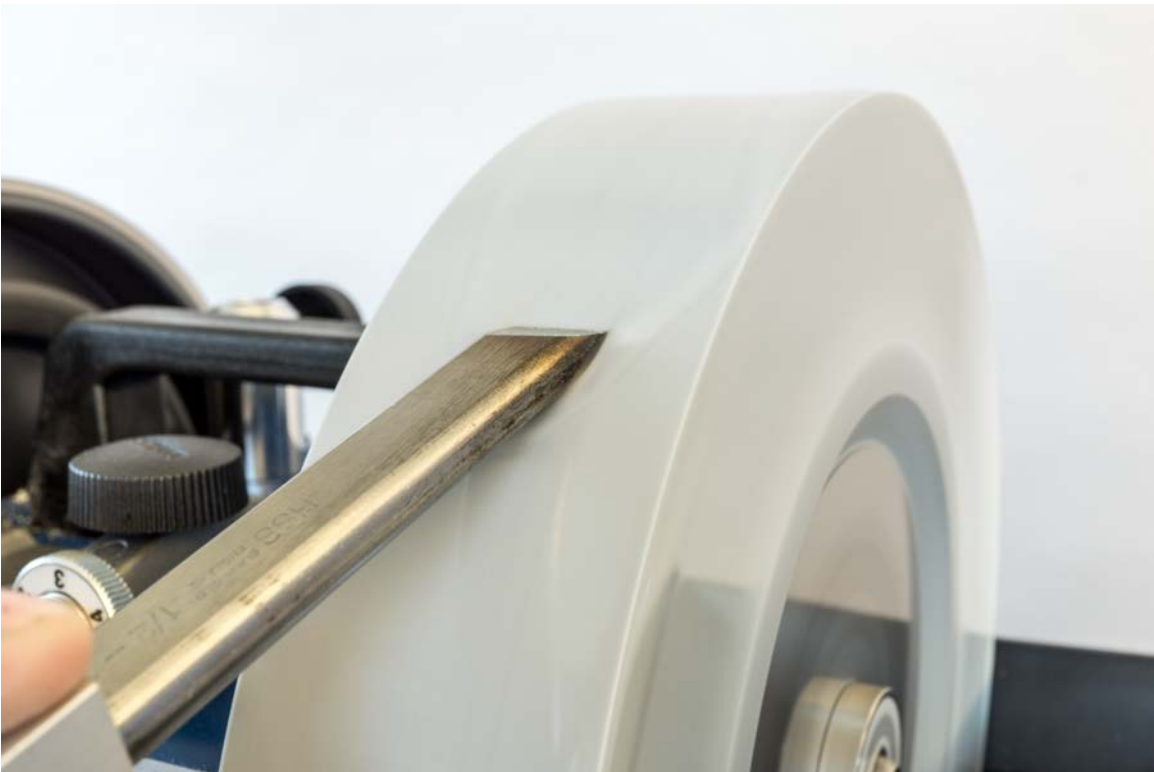
Whether a skew chisel, gouge, or special grind turning tool, all can be accommodated with the assortment of jigs available. The keener edge cuts better and lasts longer.
