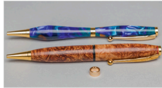
Eliminating the centerband allows you to use the basic 7mm kit, yet have size and shape freedom.
