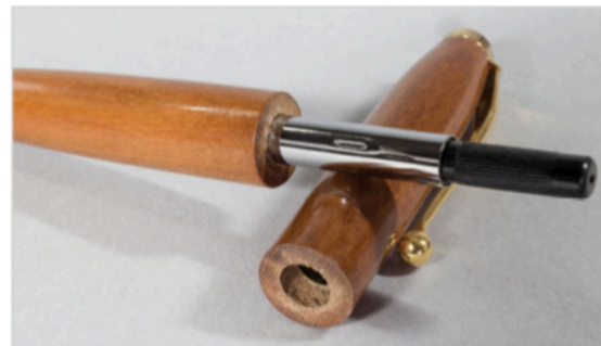
If you feel the need to make up the lost centerband length, you can easily do it by having some unsupported length in the middle.
