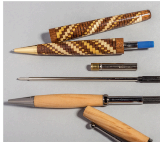
Without the centerband, you have great latitude in how long or short your pen can be. You're no longer restricted to turning to exact dimensions.
