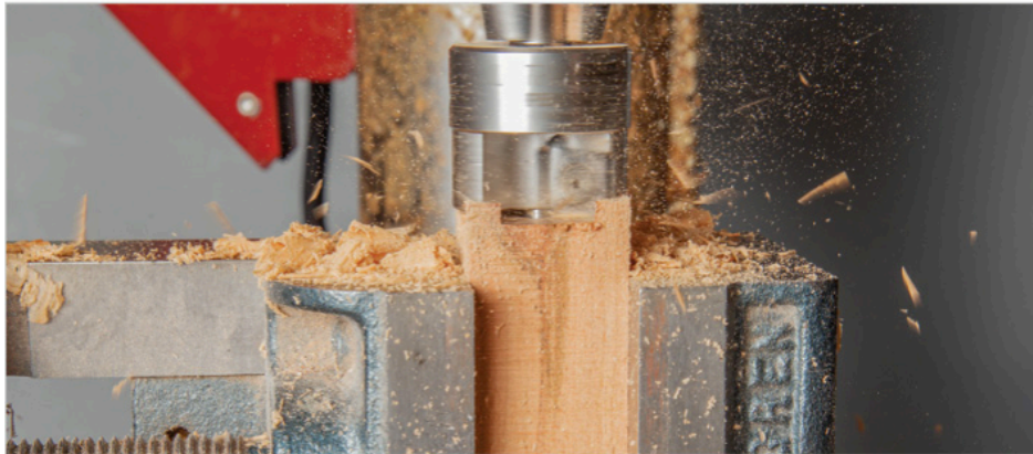
I favor the Ultra-Shear Pen Mill Ci to face my blanks. I find the control for depth and perpendicularity far more controllable with better surface results.
