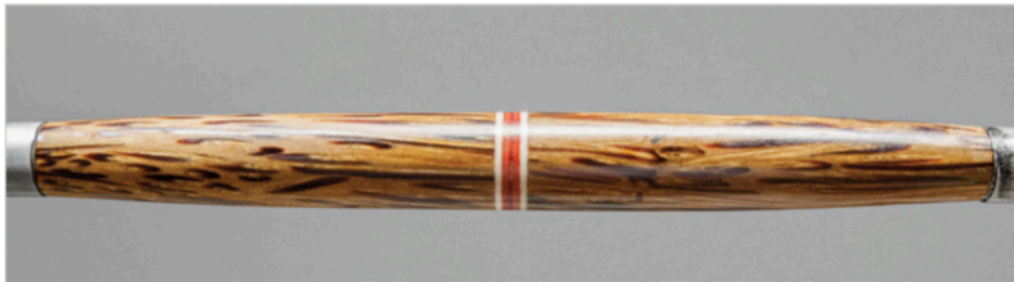
The simplicity of turning, sanding, and finishing the blanks butted together, with no center bushing in place, makes creating more pleasing shapes easier. You'll get a perfect fit between the upper and lower barrel, as well, since they're turned together.
