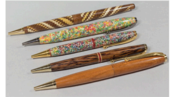
The 7mm kit can be a truly versatile building block for your turning creativity once you decide to leave the centerband out.
