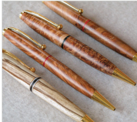
A few examples of centerbandless 7mm kits using some colored plastic for accenting. The plastic is end glued on to the barrels and turned with the blank butted together.
