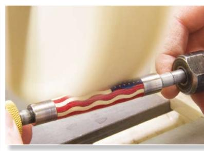
Pen parts in particular have a nasty habit of getting away or rolling off on to the floor. I find that leaving the barrels on the mandrel through the entire process makes it easier to handle and less prone to damage
