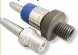
There are commercially available tapers with headstock threading for non-powered use. A non-rotating taper threaded mount can be obtained with a revolving centre by putting an Allen wrench or wooden kebab skewer into the rotating lock hole
