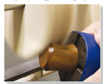
Keeping your work mounted on the workholding device often makes buffing more secure. It often provides a better grip and keeps hands out of the way. If needed, put a wrap or two of tape over any corners of concern
