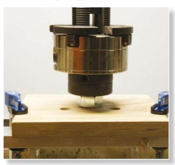
A 3/4-10 threaded bolt countersunk into a mounting block allows for use of all of my tailstock threaded fittings. Using a thread adaptor allows all of my 1-8 headstock threaded workmounting mechanisms to be used as well
