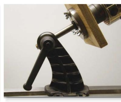
The same mounting block also has the bolt pattern and countersunk holes for easy mounting to one of my carving vises. The vise shown removed from its usual bench location. Installing a mounting base would for allow use anywhere
