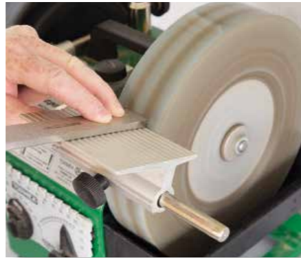
Your choice of sharpening systems can be based on the hollow grind desired and the grit of the wheel. A Tormek has about a 250mm radius and 200 grit wheel
