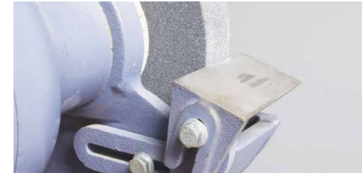
Both grinding wheels are identical at 60 grit – my choice of balance between coarseness for shaping and fineness for sharpening. The cast iron rest, which needs a wrench to adjust, is ideal for my needs
