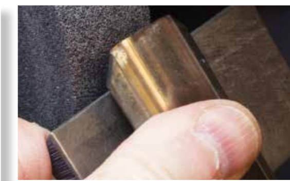
Anchor yourself to the grinder, being careful of pinch points for safety. Once you are anchored, you can put the tool on the rest and then anchor your tool to the rest for the sharpening process
