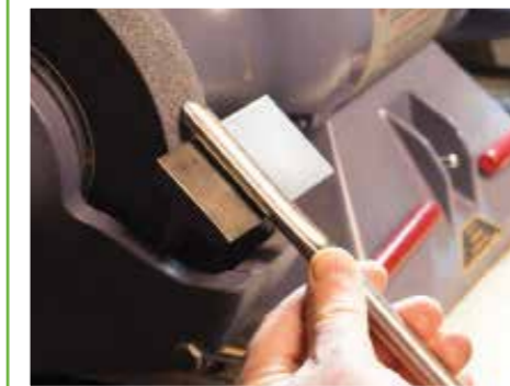
Like the fundamentals of turning, if you aren't anchored there is no way you can have good control. A common mistake is not anchoring yourself and then your tool to the grinder
