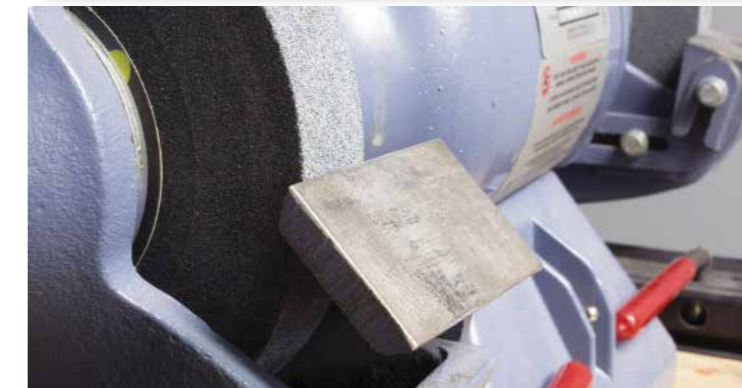
The left side set for my cutting tools at about 45° and the right side for my scraping tools at slightly less than 90° will allow me to sharpen 90% of my tools quickly, easily, and repeatedly
