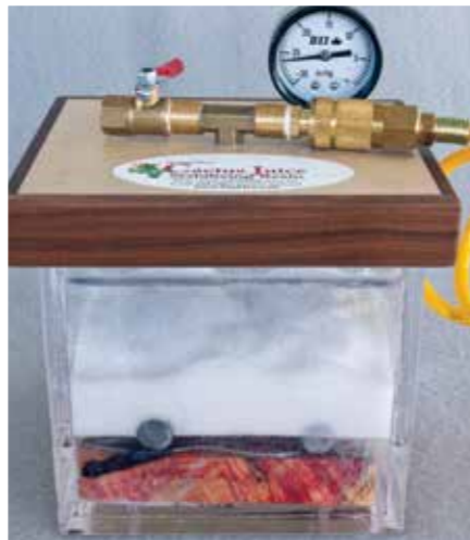
I use one of the older Cactus Juice vacuum chambers. It is clear and spec'd to 29inHg vacuum though my pump doesn't make it
