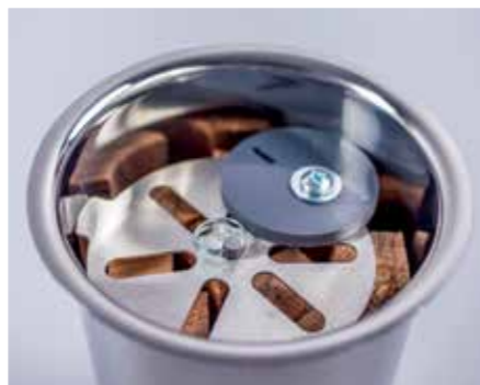
Use the smallest tank you can to minimise the need for quantity of resin to cover. Unabsorbed resin can be reclaimed
