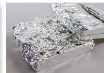
It is advantageous to keep the size of the package to be heat cured to a reasonable size. The full temperature needs to reach the centre
