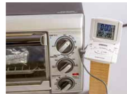
Regardless of the oven used, an accurate temperature reading is necessary. The dials are extremely inaccurate
