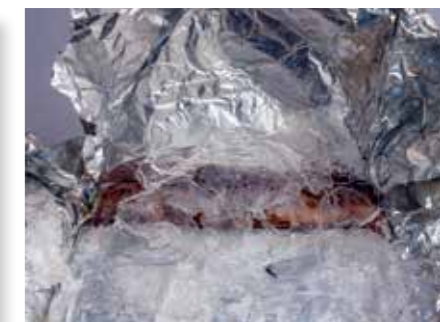
Some of the bleed out shown to illustrate the final result. The resin within the blank is turned to a clear plastic stabilising it forever
