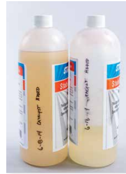
The dozen very porous blanks stabilized for this column consumed only 24oz of resin. All of the rest was reclaimed for future use
