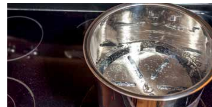
The beauty of boiling water curing is the simplicity. Easily done anywhere, inside or out, and simple stable temperature control
