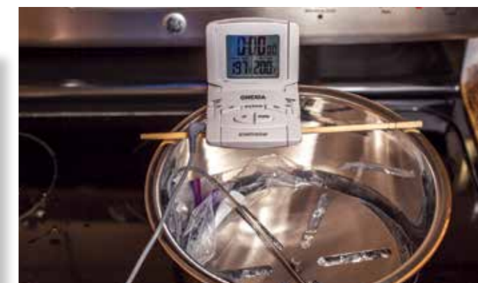
I checked my low boil temperature and found it to be 197°F. The actual will vary with barometric pressure
