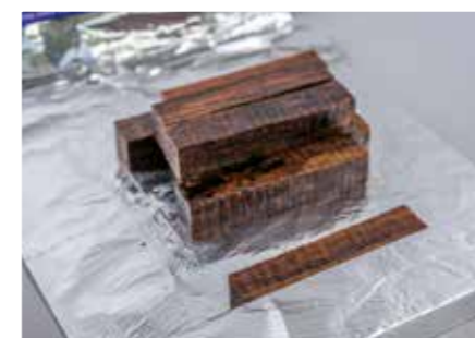
After draining, the blanks are wrapped in aluminium foil to separate them, preventing fusing together and to contain bleed out
