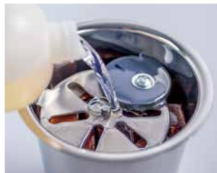
The catalysed resin is poured in to generously cover the wood being stabilised. Sufficient resin is needed to allow for impregnation
