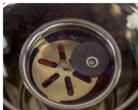
Maintain the vacuum until the rate and size of bubbles diminishes to a minimum. At that point, the vacuum can be released
