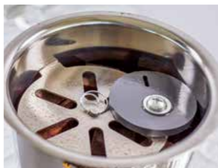
After the vacuum is released and the blanks have had their 'soak' if you follow those instructions, the excess resin can be reclaimed
