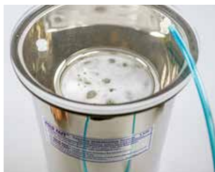
The chamber is evacuated but done slowly to prevent foaming over the rim. Use any vacuum limits per your chamber manufacturer specs
