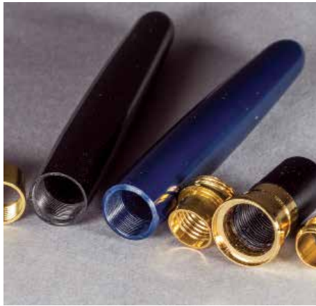
Fine pitched threads can be taken from old pens, scavenged kit parts, or other items and embedded as needed in your turnings
