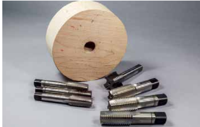
Woodturning retailers usually have the headstock and tailstock taps, which allow for direct mounting of work or making fixtures
