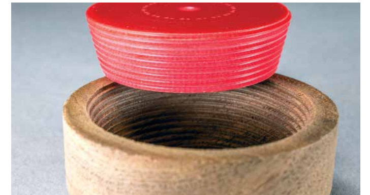
You may have immediate need for tapered threads, but hand chasing allows you the capability to cut any size and angle you wish
