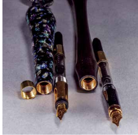
Using kit parts made the custom pens possible. The metal threaded sleeve was embedded allowing for thin walls with strength
