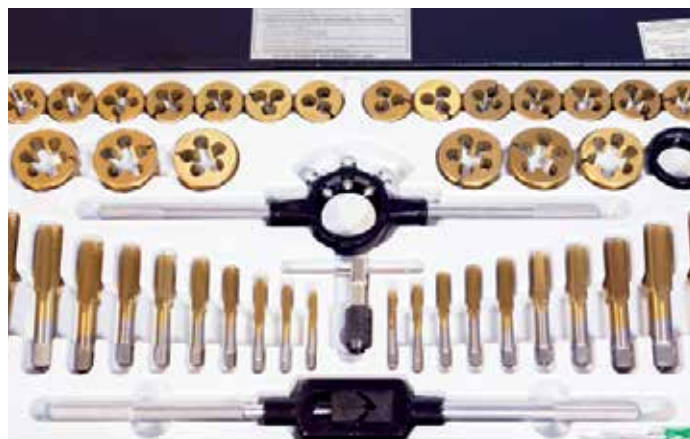
The very inexpensive tap and die sets are available in metric and unified. They will be more than serviceable in wood
