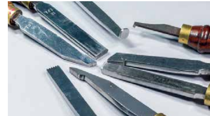
Learning to hand chase threads in wood is not difficult. The huge advantage of hand chasing threads diameter independence
