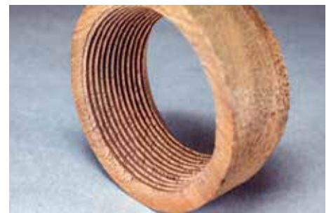
Faceplate orientation cut threads also have challenges. The fragility based on grain orientation along with roundness changes
