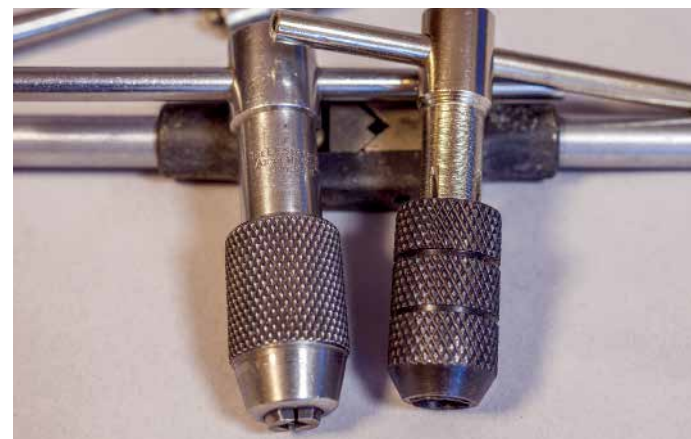
While the kit contents aren't Starrett quality, they will work well. You usually use the chuck in the lathe and hand turn
