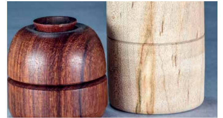
One of the challenges of threaded tops and bottoms is making the grain match. There are some tricks for lidded boxes
