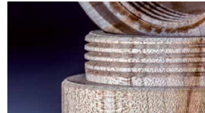
One way to improve thread life in softer woods is to not cut the threads to a sharp peak. Leaving the thread flattened will help
