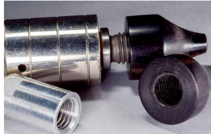
My tailcentres all have a 3/4-10 threading, allowing me to make many tailcones, mandrel savers, adaptors and hold 6mm shaft items
