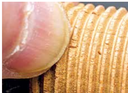
Even without sharp 'V's on the threads, wooden threads are very vulnerable to damage
