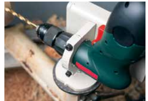
Handy for drilling holes on a lathe, a drilling fixture provides angle setting, depth control, and rotational position when used with the lathe indexing lock
