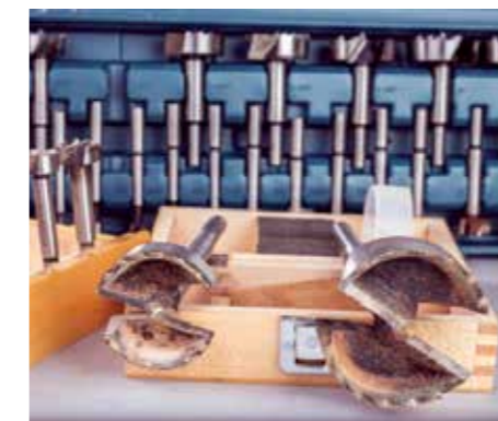
Sawtooth bit sets are available at very modest cost. Larger or speciality sizes are usually quite expensive
