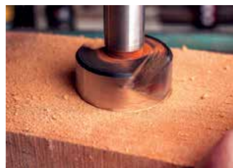
Very effective for clean entry in face grain, the outer perimeter scoring cutters engage after the pilot point and just before the peeling cutters
