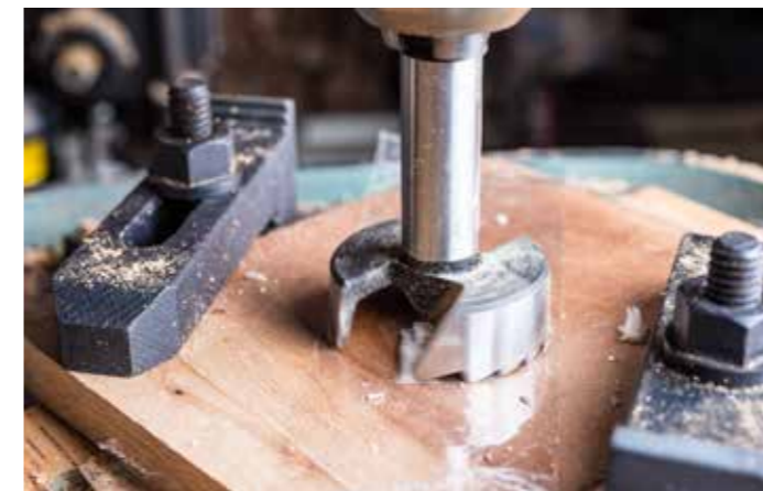
A thickness of packing tape on the top and bottom surfaces seems to help minimise damage as does always having a sacrificial breakout backing block. The piece is clamped down to prevent spinning if jamming of the blade occurs
