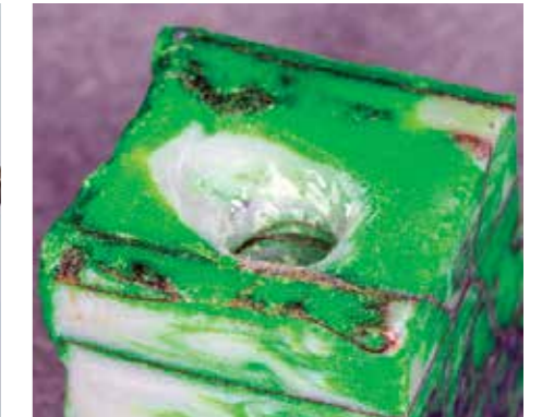
Rare in woods, blow out at the exit is common in brittle plastics. The easiest solution is to leave sufficient stock for cutoff to the unaffected area
