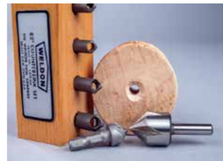
Even the most modest priced countersink will do a better job of a chamfer than attempting to use a twist drill as this turner did
