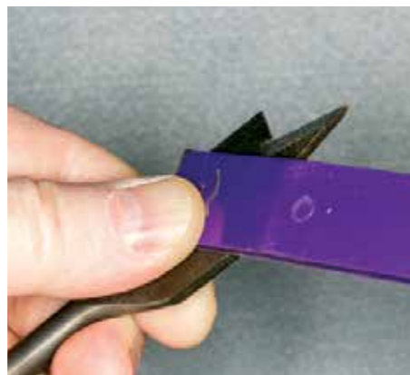
A diamond hone can sharpen a spade bit nicely, used in the same fashion as for a sawtooth bit: flat on the surface leading to the cutting edge on both sides
