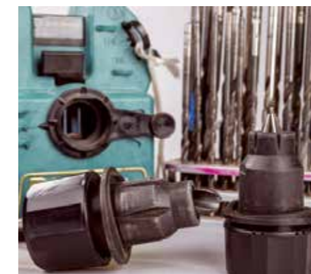
My drill sharpening machine sharpens 118° and 135° drills from 2.38mm to 19mm quickly and repeatably
