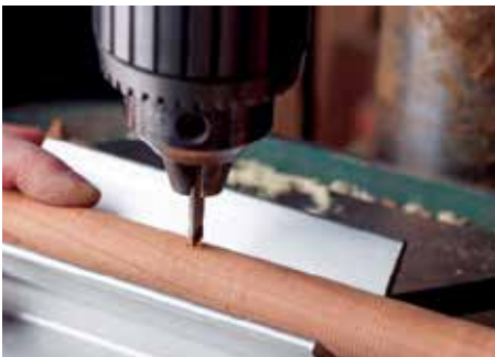
When drilling round stock in a drill press, always use a 'V' block to safely hold the work and a centre drill to spot your starting location
