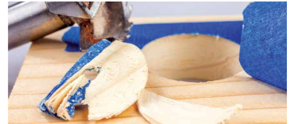
The exit hole in softwood shows the tape used to assist with the process. Force reduction just prior to breakout will allow for the breakout to be a clean 'plug'
