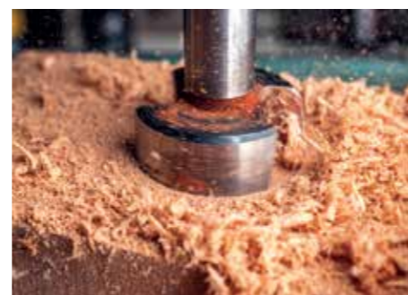
With the scoring cutters leading the way, the peeling cutters can act just like a bench plane when drilling into face grain
