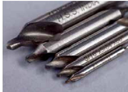
Very rigid and short, especially the drill portion, machinist centre drills are used to create the starting point for your subsequent drillings. It prevents wandering
