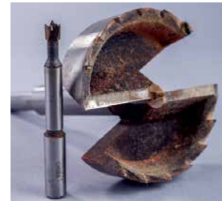
The surface feet per minute of the cutting edges at the same RPM is quite evident between a 6mm and 80mm sawtooth bits
