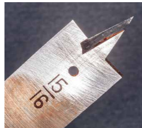
Even with the OD edge of the blade engaging first, a spade bit is a scraper and is brutal on the entry and exit hole surface finishes. Avoid using them in woodturning
