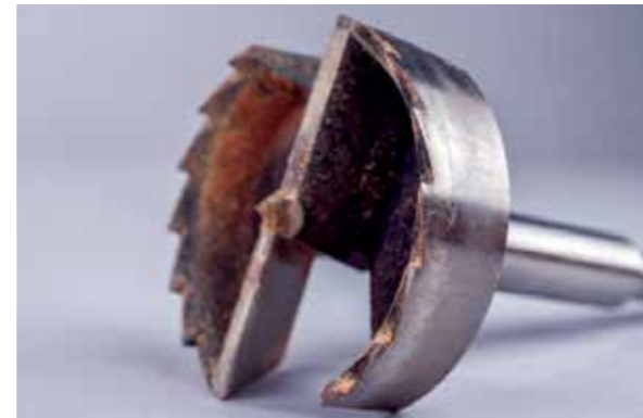
The outer perimeter scoring cutters perform valuable work on face grain. Most turners should never attempt to sharpen them
