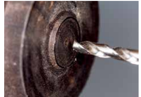
Using a centre drill to create the starting point, even a long, slender drill, such as this 3 x 150mm will start exactly where desired
