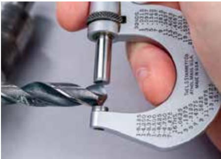
The true size of a drill is the measurement across the cutting flutes. It isn't the stamped size or the shank measurement. When important, measure a drilled test hole
