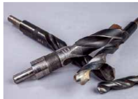
When drilling larger sized holes, it is often better to start small and do progressively larger drilling rather than attempt a single large hole in one pass
