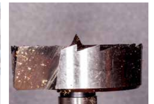
A sawtooth bit does three functions in sequence: the centre point provides guidance; the scoring perimeter slices the face grain and peeling cutters slice the material out
