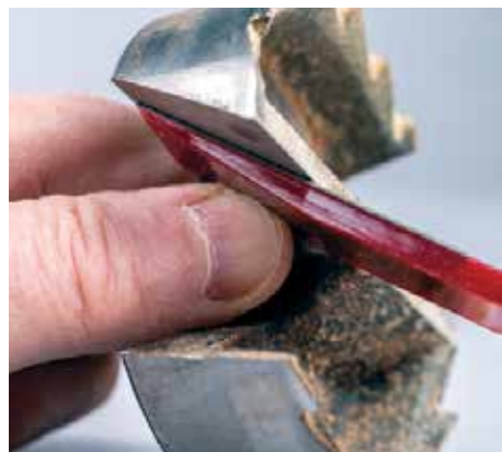
A diamond hone held flat to the front surface leading to the peeling cutter edge while sliding the hone back and forth will help keep your sawtooth bits sharp
