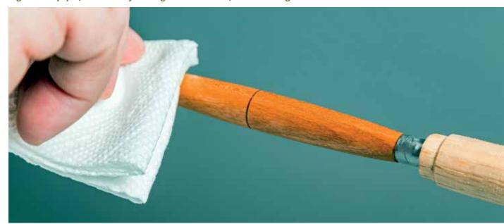
My method for CA application is light coats of thin CA wiped on axially end to end incrementally, indexing the headstock by hand at end of each wipe
