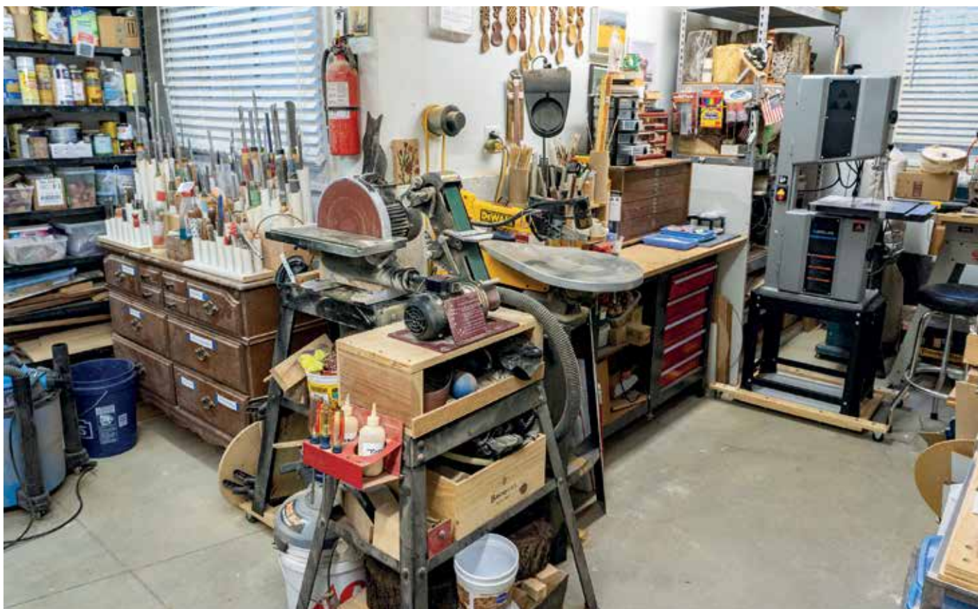
Natural lighting available, reflective wall colouring, equipment on mobile bases, and moderate-sized machinery make maximising space and flexibility possible
