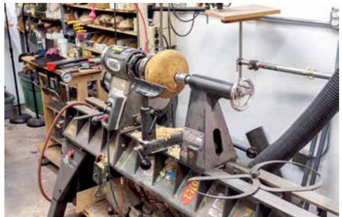
White or near-white walls spread light and provide great backdrop contrast to turnings. When black is desired for whiter woods, a piece of dark coloured Masonite can be placed behind the machine
