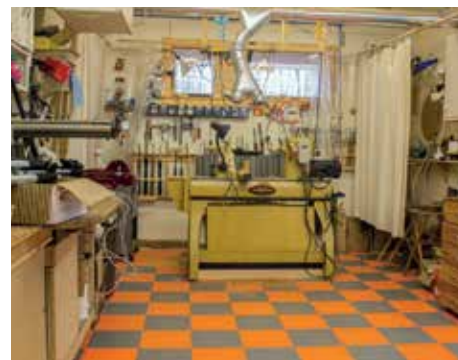
New building planning is a good time to adequately size dust collection and route the system to minimise losses while providing connections as needed
