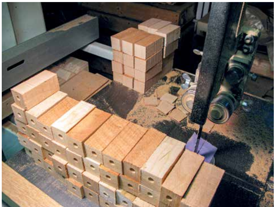
Set up your process to work in efficient sized batches. You don't need all 250 blanks sitting in a pile waiting for turning. Only enough to keep ahead of the turner. (My prep for upcoming classes)
