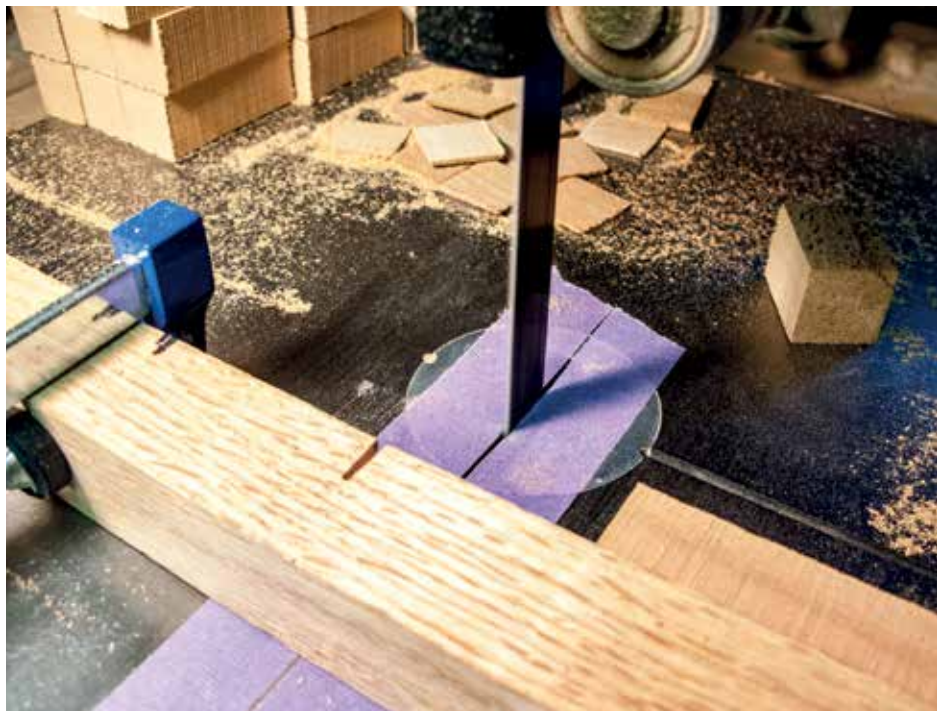
Jigs and fixtures can be as simple as setting a proper length cut off clamp on the bandsaw. Set it for minimal excess needed for barrel trimming, and yet a non-turner can process blanks
