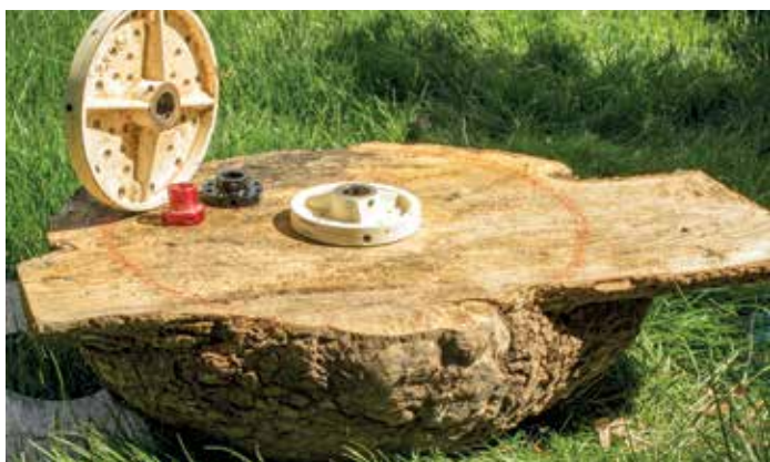
Faceplates, in various sizes, excel for mounting and turning larger blanks. With proper faceplate sizing and mounting screws, they allow safe turning of many different blanks
