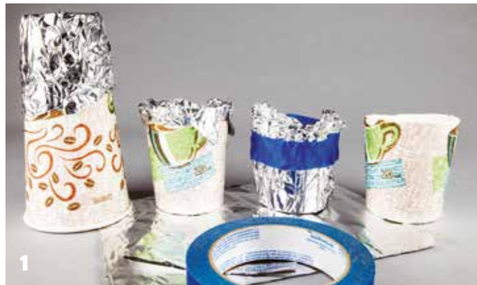
1 A cup (or whatever) used as a form, that formed foil mould as a liner, a standalone mould reinforced with some tape, and a sacrificial mould (after testing for inertness) of the desired size 2 No need to remove the foil mould from the casting. Continue to process your blanks as if it wasn't there
