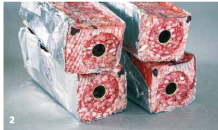
1 A cup (or whatever) used as a form, that formed foil mould as a liner, a standalone mould reinforced with some tape, and a sacrificial mould (after testing for inertness) of the desired size 2 No need to remove the foil mould from the casting. Continue to process your blanks as if it wasn't there
