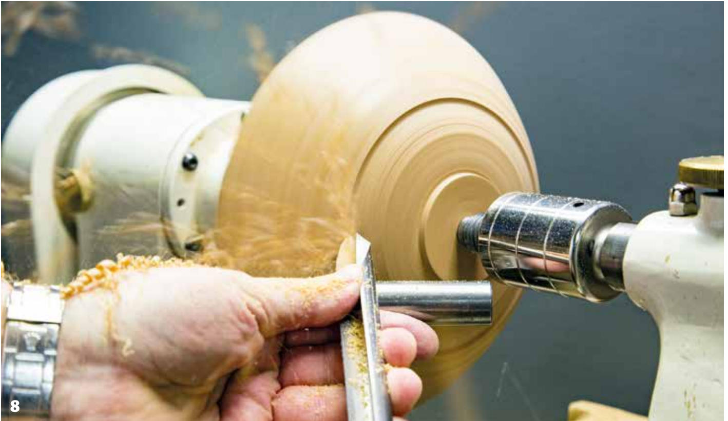
6 The ability to put a quality cutting edge quickly and efficiently on your tools is a skill that is key to your skills growth in woodturning 7 With some additional grinding skills, you'll be able to not only grind a well cutting edge on your tools but also be able to quickly determine its state with a look and feel 8 Your cuts will be better quality and require less effort with a properly sharpened tool. With experience, you'll be able to feel the need for a touch up as you cut
