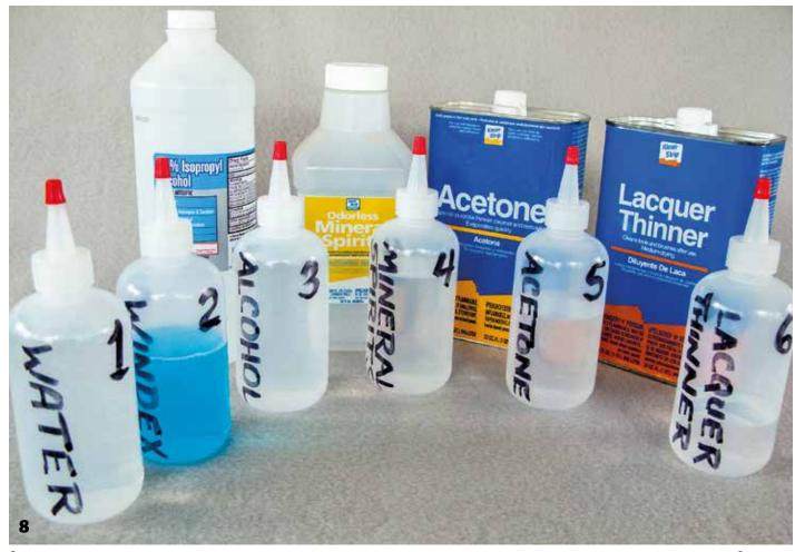
**8** A handy shop tip for solvents is to have small chemical bottles with the six most-used solvents, in order of aggressiveness, already decanted and ready for use **9** Be certain any transfer bottle is clearly marked with the contents. I keep this plastic tote handy for use right at the lathe. Precise dispensing and then capped
