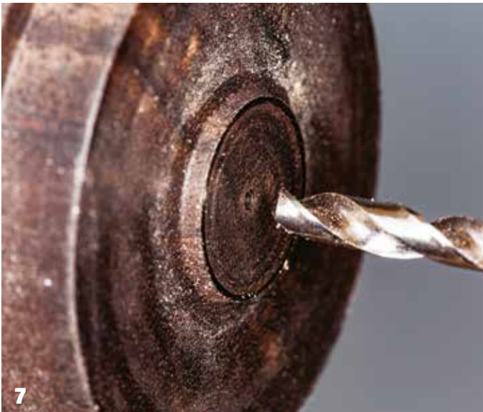
5 It is key that a starter location be created for any off-perpendicular drilling. A starter location is critical for safety and success 6 Holes for a double strand of 2 or 4lb. test fish line are in the .038in arena. You can break a lot of small drills if you don't work carefully 7 Even a perpendicular, flat surface benefits from a starter drill location. Only taking moments, this 1/8in drill will have no location or starting issues 8 With a good starter drill location, a sharp drill allowed to do the work can be hand held to drill small holes quickly.
