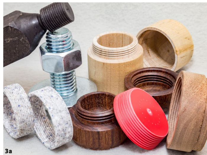
1 Matched sets, male and female, are available in a variety of thread pitches. With those two tools, you can cut threads. 2 Learning to chase threads is a great skill to develop. Not a necessary skill but certainly expands your repertoire. 3a & 3b Tapered threads, insertable thread pairs, standard mating threads, in wood and plastic. Pair diameters limited only by your lathe.
