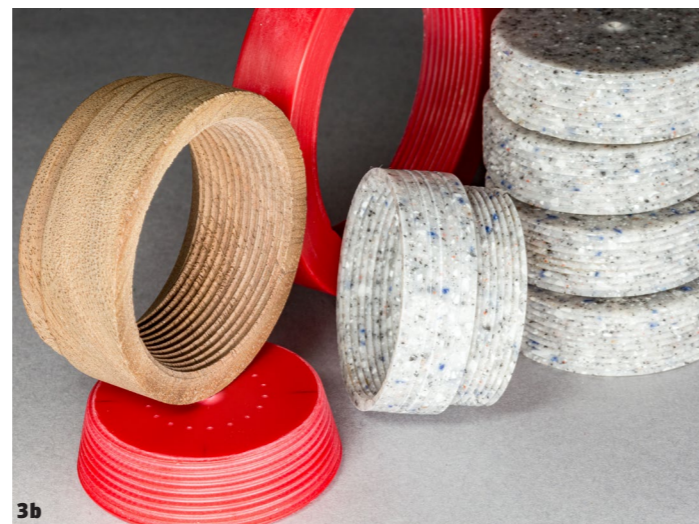
1 Matched sets, male and female, are available in a variety of thread pitches. With those two tools, you can cut threads. 2 Learning to chase threads is a great skill to develop. Not a necessary skill but certainly expands your repertoire. 3a & 3b Tapered threads, insertable thread pairs, standard mating threads, in wood and plastic. Pair diameters limited only by your lathe.
