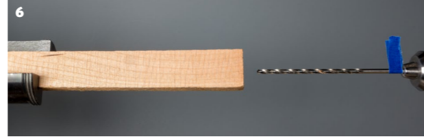
1 Large or small drills, I use a technique learned from Dick Sing. With the quill retracted, slide the tailstock forward by hand to drill your hole. 2 Keeping your drills sharp is key to good holes. The best investment I have ever made for drills was an inexpensive sharpening machine. 3 If you do purchase a sharpening machine, be certain you can sharpen the range of drills you use. 4 Many times, issues with concentricity or other drilling related issues are workholding related. Get as much of your stock mounted well. 5 Good drilling practice, using proper speeds and feeds, includes retracting the drill and cleaning the flutes as needed. 6 An 1/8in, 5+ inch deep drilling on an unsupported blank presents problems. Notice the grain orientation that may take over the guidance to a degree.
