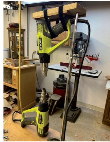
4 Sometimes Bruce draws a piece he's going to make on a drafting table 5 He frequently sketches an idea on an iPad 6 Heat guns set up for bending plastics. Heating from the top and bottom provides an even distribution on the plastic 7 (Below) The 3D pen he uses including some different filaments (below the pen)
