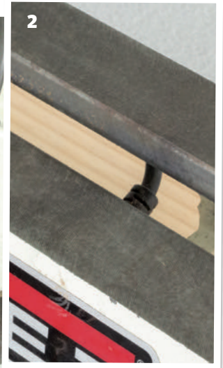
1 The mechanics of clamping the banjo and tailstock in place. Even with the much more effective homemade clamp block on the tailstock, a rusting of the ways works wonders 2 You don't need pitting or extensive rusting. A slight rusting will add sufficient friction to allow for normal tailstock clamping forces
