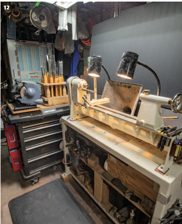
10 My main shop has very little natural light. Each workstation has equipment-specific lighting installed. This lathe has two 4ft, double lamp LED lights directly over the bed 11 For task lighting, I have two gooseneck lamps installed to the lathe. Not only moveable because of the gooseneck, but also relocatable on the lathe 12 A look at the set-up of my lathe in my main shop. With the overhead lighting and the lathe-mounted gooseneck lamps, I usually have plenty of light for most turning 13 When the situation requires more light, often up very close, I can bring one or more of these additional lamps to bear. There are also clamp-on lamps if needed 14 Natural lighting is wonderful if you have windows or doors near your lathe. With open doors, you sometimes get unexpected visitors. Here, Cholo looks around
