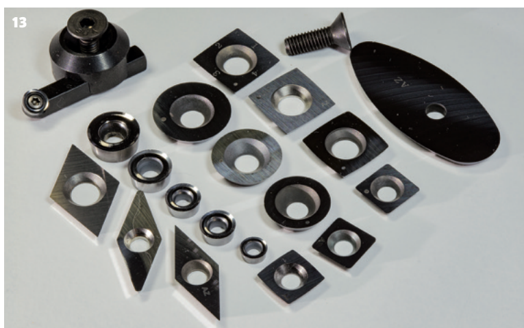
13 Just a small sample of the carbide cutters now available for woodturning tools. Many of these cutters will create curls as compared to the traditional machine tool cutters.
