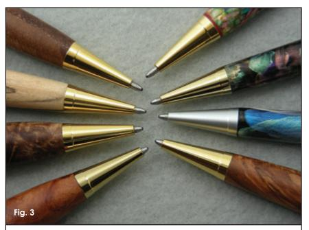
From the too short to the obviously way too long tip extension. Take the time to use the intended inkfill to do the press in the assembly of your pen.
