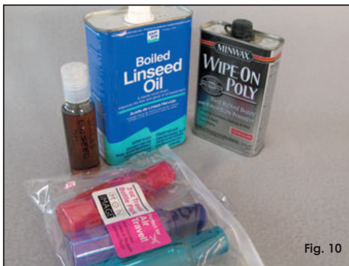
Decanting chemicals and finishes into working-size containers is much more convenient for use in the shop.
