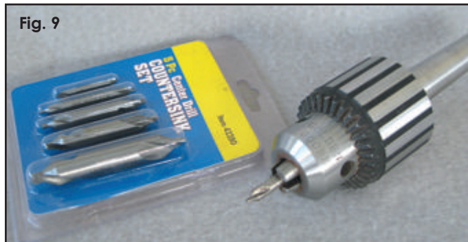
A center drill, used in a drill chuck, is a great way to start drilling in the lathe.
