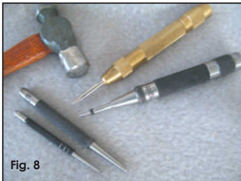
Giving your drill a good starting point is easy with one of the spring-loaded center punches or the old-fashioned prick punch and hammer.
