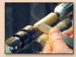
Going around a curve requires a simple rotation of the tool, while continuing to keep "forcing" the tool into the cut.
