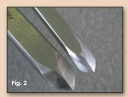
A view from the bottom side shows that the cutting edges are angled at about 45° with the bevel ground convexly.
