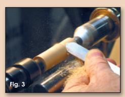
In use, the tool is presented perpendicularly to the axis of the work with the angle of the edge automatically presented at 45°, regardless of left or right direction of cut.
