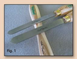
The V-skew is nicely made and is available in two sizes from Packard Woodworks.
