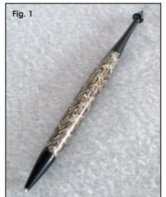
Pictures, like snakeskin, are bonded to the brass tube and then the polyester resin is cast ground it.
