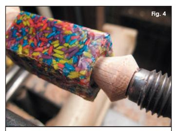
The wooden tapered plugs work nicely to center the work of any diameter tube.
