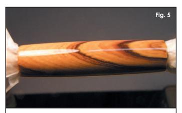
I use these wooden plugs covered with a small piece of waxed paper to allow for "no risk" CA finishing.
