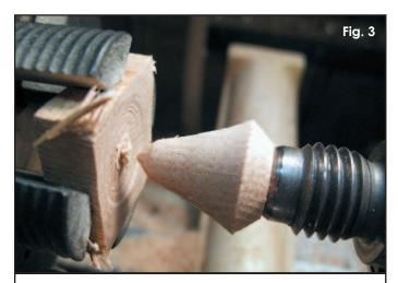
It is easy to make tapered plugs for the headstock and tail center that will center any diameter tube for sanding or finishing.
