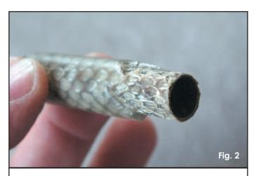
A light touch and sharp tools are absolutely key to being successful with any materials bonded to the tube under polyester resin.
