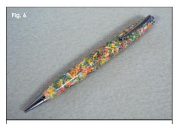
Fillers used under polyester resin may need to be end-sealed where the material breaks out during cutting. CA or lacquer works nicely if you feel the need.
