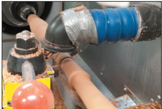
Fig. 9. The metalworking and woodworking production equipment is CNC controlled, such as this lathe that is turning one of the easily recognized EWT handles.
