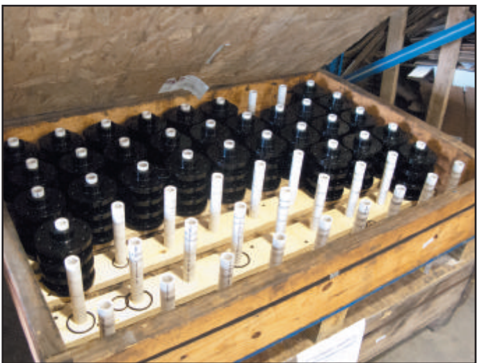
Fig. 13. Faceplates were a recent addition to the EWT product line. Here is a batch that has come back from black anodizing.
