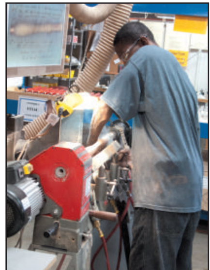
Fig. 10. Even with automation, there are some things that are best done with skilled hands, such as sanding each of the tool handles prior to application of the finish.
