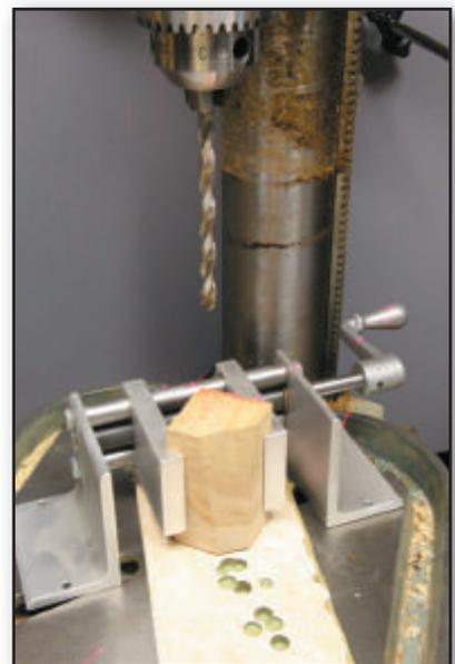
With a 1" space underneath the jaws for a drill-through block, the vise works nicely for odd shapes encountered for wine stoppers, as well as the more regular pen blanks.
