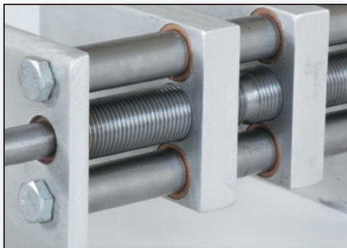
It is a quality made product with oillite bushings, cleaned-up edges and holes, and quality hardware.
