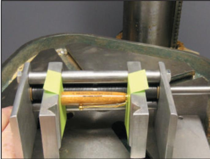
**The vise works nicely as an assembly tool with 3-1/2" between the platens. Here I've inserted some Post-it note paper as scratch and mar protection for the pen parts.**
