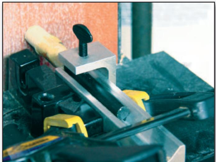
**With the platen and fence aligned for perpendicularity, the sanding block clamped to the fence will allow the user to quickly and accurately sand the pen blank back to the brass.**
