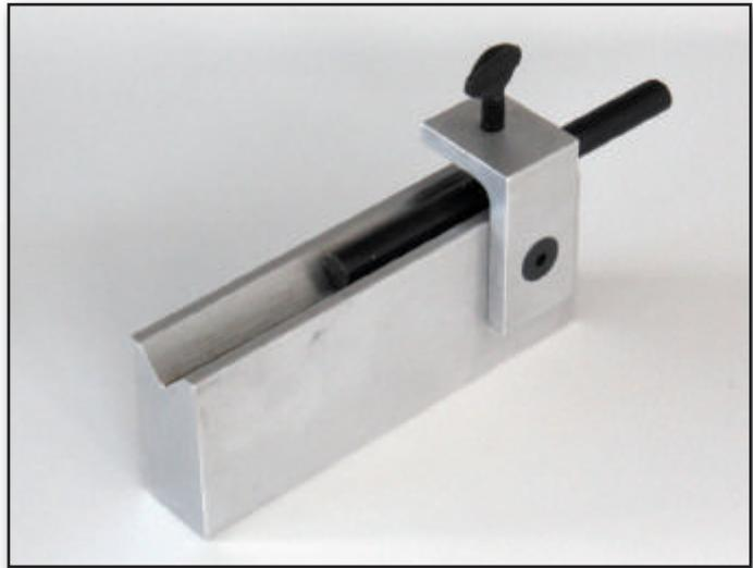
**The sanding block is designed to clamp the proper punch or dowel, allowing for the ID guidance of the pen blank being perpendicularly sanded to the glued-in brass.**
