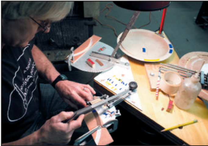
Fig. 11. The Inlay Razor is shown in action with Geoffrey cutting pieces for his current design. Much of the fun is the conceiving of unique designs along with the cutter creation and individual piece cutting.
