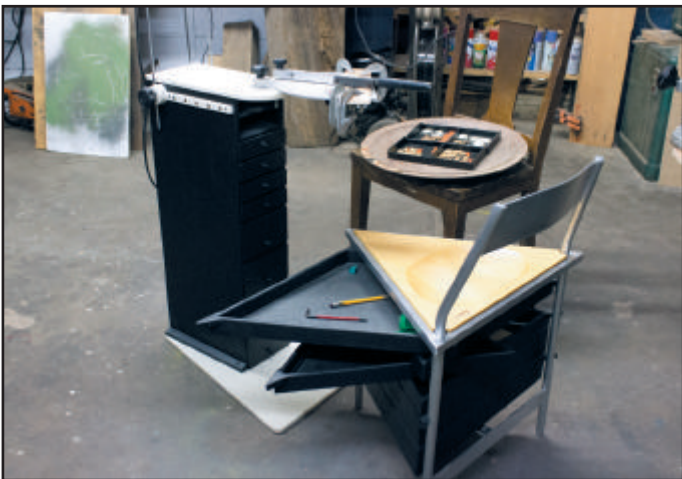
Fig. 12. Not a currently marketed product (but still a very clever idea), his workstation allows for plenty of material storage in rotating drawers in the chair and under the worktable surface.
