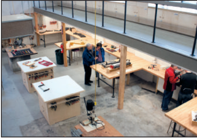
Fig. 11. In addition to the power tools available on the floor, there is plenty of bench space for layout, handwork, and assembly. The entire shop has great lighting, including plentiful natural lighting.
