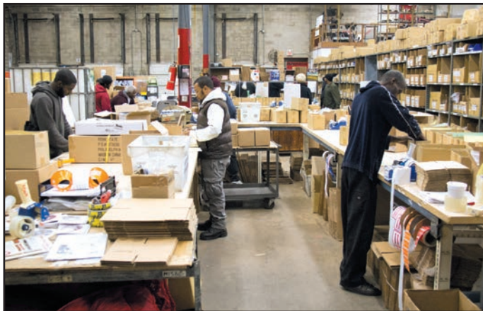
Fig. 8. The order fulfillment department picks and packs orders for daily pickup by UPS. The most commonly ordered items are placed in the storage areas immediately adjacent to the packing area.
