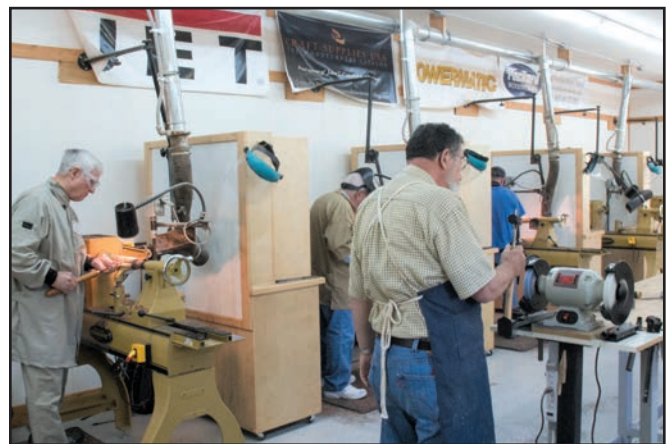
Fig. 5. The Willard C. Baxter Woodturning Studio is equipped with workstations for ten students plus the instructor. The equipment includes eleven Powermatics, eleven mini-Jets on stands, and all the shop support equipment from drill presses to bandsaws and grinders.
