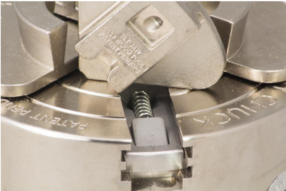
Figure 10 - With the jaw removed, you can see the locking dog returned to the locking position under spring load.
