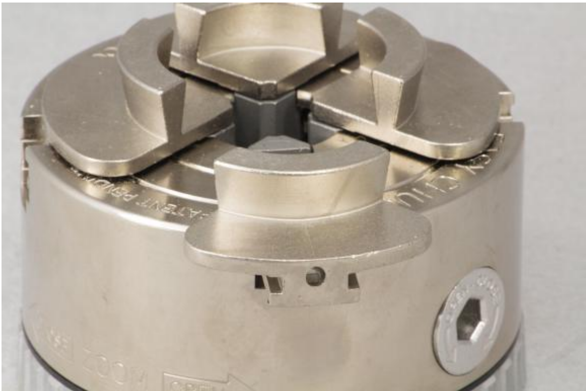
Figure 9 - With the jaw released from the locking dog, the jaw release tool can be removed and the jaw easily slide out of the chuck body.
