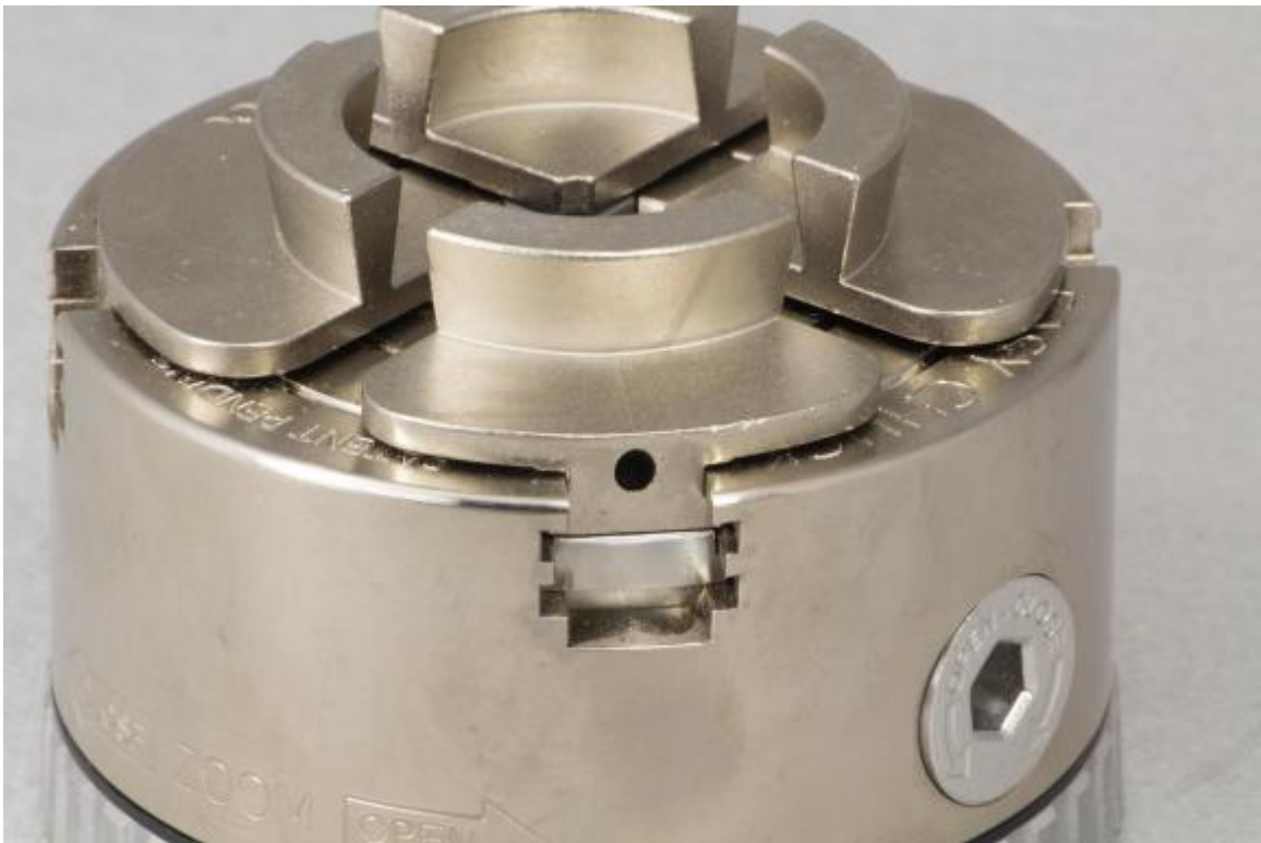
Figure 12 - The locking dog cams out of the way against the spring until the jaw is inserted far enough and the locking dog snaps into place. The jaw is locked in place and ready for use.
