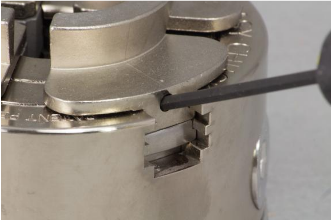
Figure 6 - The provided access hole allows the jaw key to be inserted. The jaw key, a handled ball end 1/8" hex driver doubles duty as the grub screw adjustment tool
