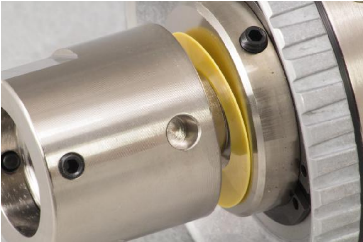
Figure 15 - The adapter is provided with spindle washers for both ends along with its own grub screws for fastening to the 1 1/4" thread.
