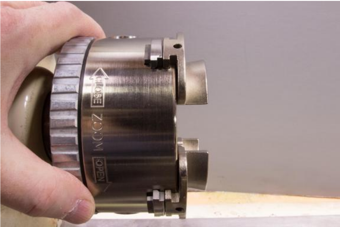
Figure 20 - The quick adjust ring makes large transitions in size a snap. Simply grab the ring and twist the appropriate direction to open or close the jaws quickly. Locking the headstock allows for easy one hand use. Jaws full open to jaws full closed is slightly less than two and a half rotations of the quick adjust ring.
