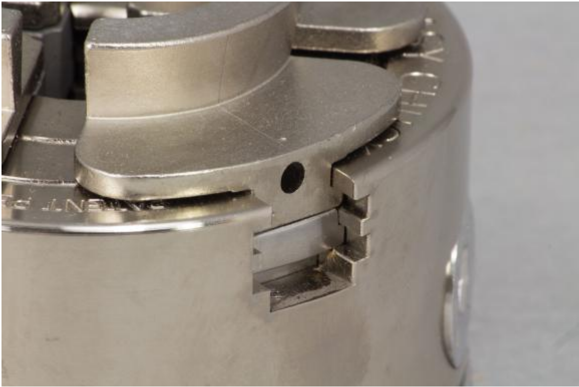
Figure 5 - No screw holes in the face of the jaws to fasten the jaws to the chuck. Only a small access hole on the back of each of the jaws.
