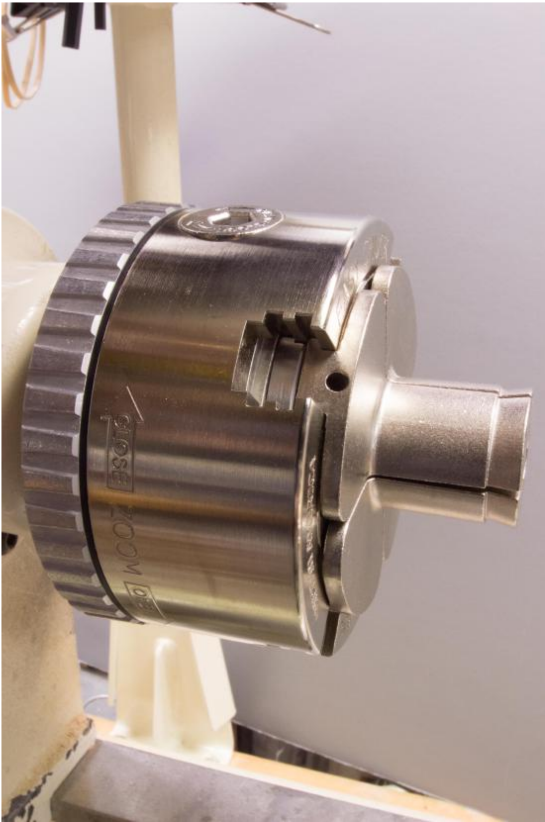
Figure 23 - The other extreme in jaws is the "B" Easy Reach Dovetail Jaws. Both internal and external dovetails along with a 1 1/4" jaw length.
