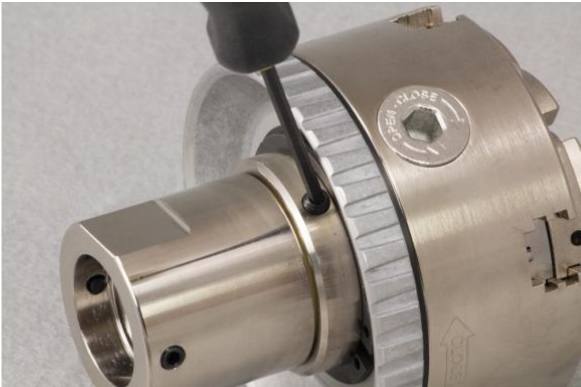
Figure 17 - The ball end hex key used as a jaw release tool does double duty to tighten the grub screws.
