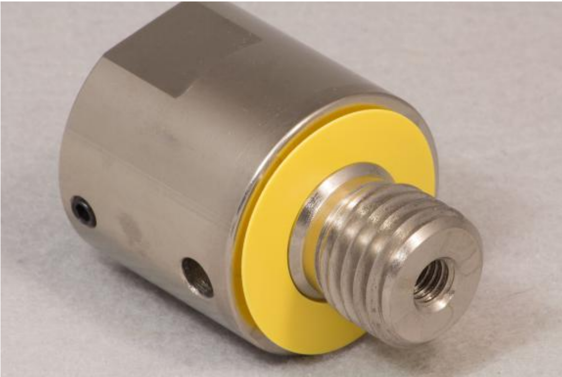
Figure 28 - A thoughtful touch... Threading the adapter for 3/8" - 16. The same thread as most of the bottle stopper threads.
