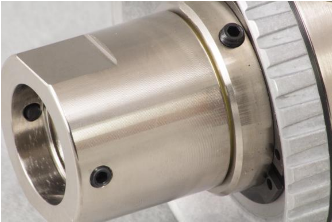
Figure 16 - The adapter has both machined flats and a breaker bar pocket should things become too tight and need some “coaxing” to be loosened. Shouldn’t be required too often if you use the spindle washers and avoid horrific catches that tend to tighten things up.
