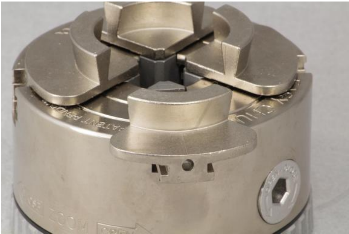
Figure 11 - To install a jaw, it is simply slid into the channel and pushed forward.
