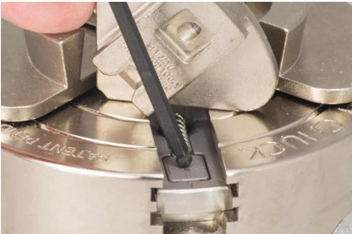
Figure 8 - It presses the locking dog down against the spring load allowing the jaw to be released by sliding it slightly outward.
