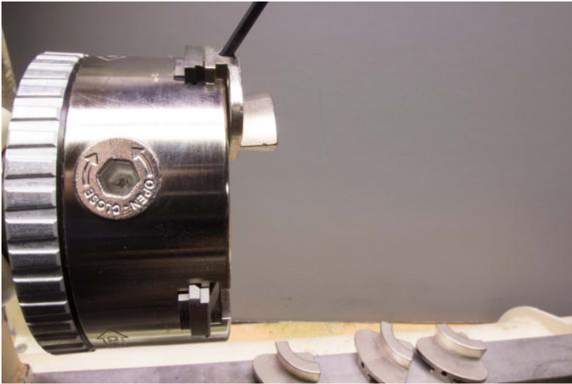
Figure 21 - No screws to worry about when changing jaws. One simple tool slid into the hole and the jaws are easily removed. Fifteen seconds total to do a complete jaws change if you are dogging it.
