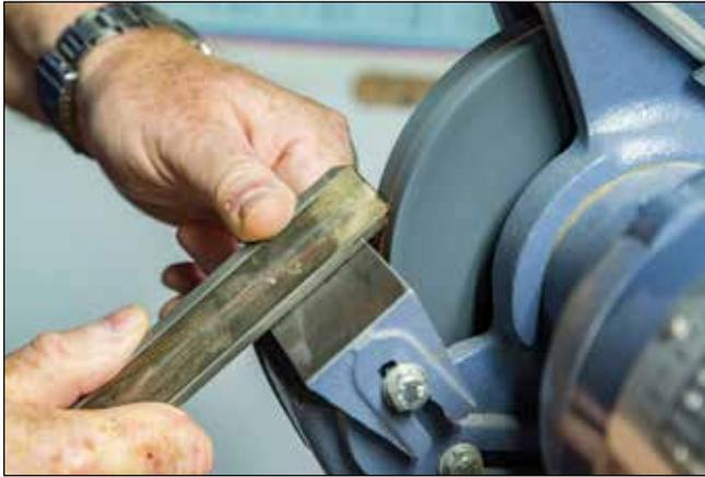
**Toolrests** – The toolrest needs to be positioned correctly and rigidly to provide a stable and repeatable platform. It should be large enough to support long turning tools yet small enough for short tools, too.
