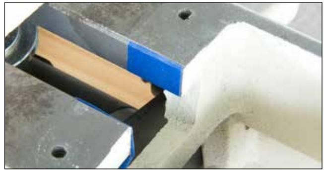
**Shims** – For height or tilt misalignment, add shims made of tape, foil, or paper. It’s also possible to file the bolt holes a bit larger, and to file the machined surfaces on the bottom of the headstock.
