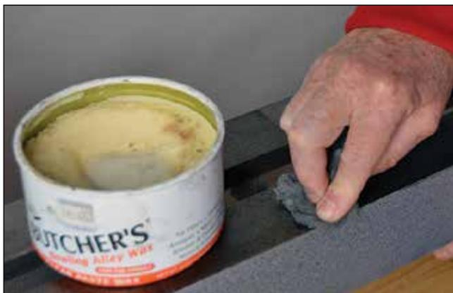
**Wax it** — Waxing the ways prevents rust and helps the banjo and toolrest slide smoothly. Your lathe may also benefit from filing any dangerously sharp corners, edges and burrs.
