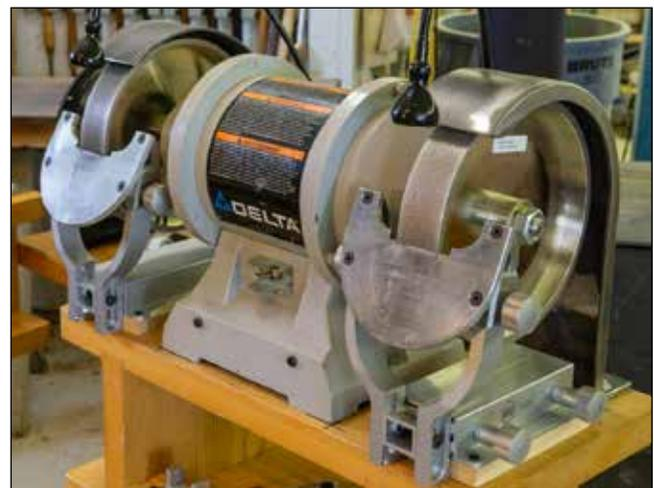
**Bolt lock** – High-end setup has CBN wheels with robust bolt-locking guards, adjustable tool platforms, and bright task light.
