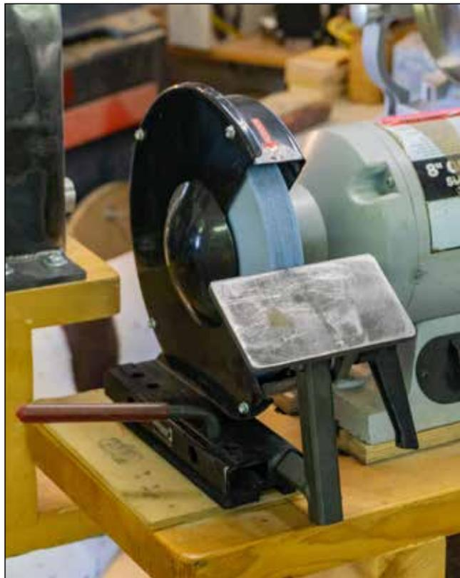
**Adjustable** – Good setup has grindstones mounted at proper height, interchangeable toolrests that lock in place, and safety covers.
