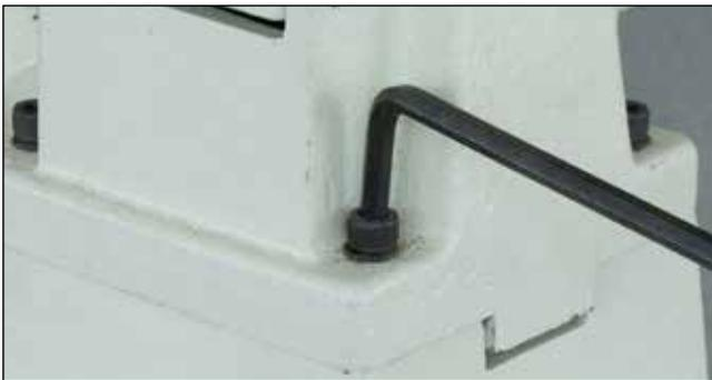
**Headstock** – Sometimes it’s enough to just loosen the headstock bolts, shift within the hole tolerances, and re-tighten. Note the slop in how this headstock fits the lathe bed.
