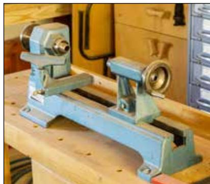
**Bench** – Small lathes may be just right when bolted to a workbench; adjust upward with blocks, or “downward” by standing on a mat or low platform. As little as 1/4” (6mm) can make a discernable difference.
