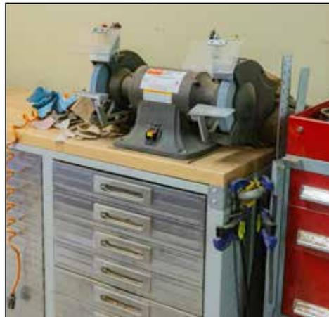
**Bench** — Mounting the grinder on a bench secures it from sliding and provides storage for accessory fittings.
