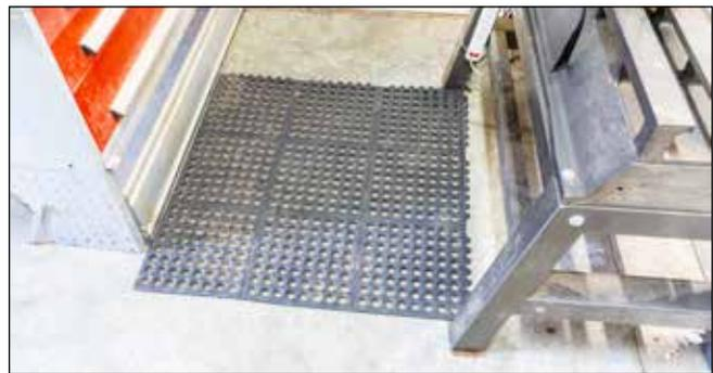
**Floor mats** – Standing at the lathe tires you out. Anti-fatigue mat intended for food service has flexible spacing dimples and large holes for easy cleanup. Mats designed for shipping fragile high-end electronic assemblies are expensive, but very comfortable, below.
