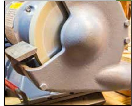
**Sturdy** – A properly installed end shield still allows plenty of access to the side of this CBN wheel.
