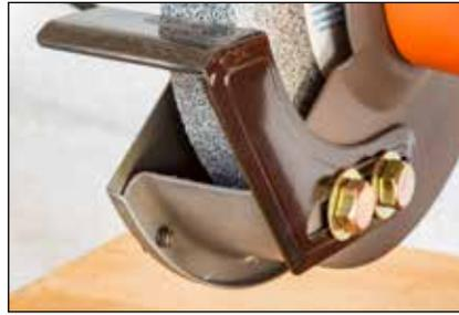
**Flimsy** – Cheapo grinders have small, flimsy toolrests and wheel shields.
