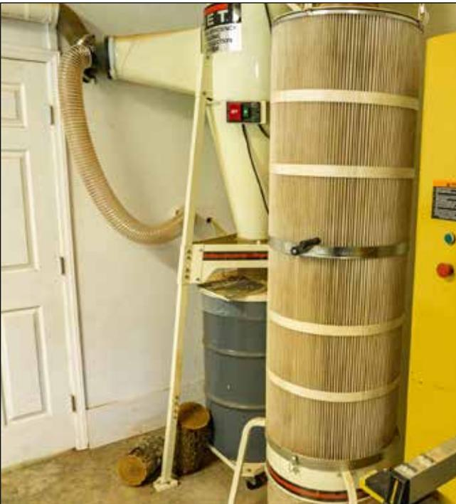
**Noisy machine** – Locating the dust collector outside the workshop reduces noise and exhausts the unfiltered small particles away from the turner.
