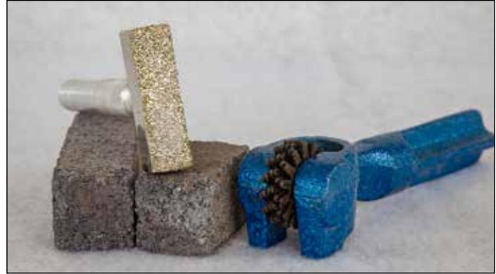
**Wheel tools** – Grinding wheels can be flattened and cleaned with a devil stick, a star wheel, or a diamond dresser.
