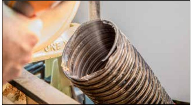
**Not fancy** – The bare vacuum hose extracts a visible plume of sanding dust. There are many different designs for dust hoods. You won’t intercept it all, so also wear appropriate personal protection, a dust mask or filtered-air faceshield.
