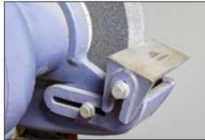
**Solid** – Cast iron rest has a large platform and bolts securely in place.
