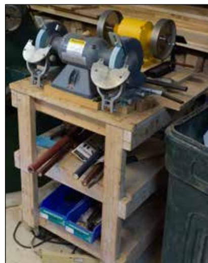
**Shopmade stand** — The right height depends on the turner's height. You can make a sturdy stand from 2x4s glued and screwed together.
