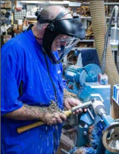
**Right height** – The turner can stand upright and present the tool comfortably. This helps with back fatigue.
