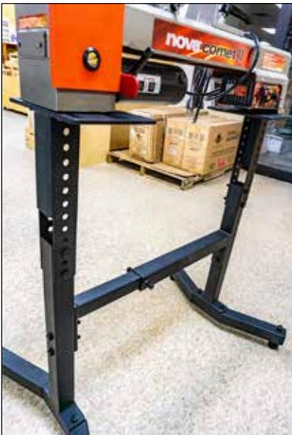
**Adjustable stand** – Many manufacturers offer an adjustable stand for their lathes. Also available are generic adjustable stands capable of fitting virtually any mini-lathe.
