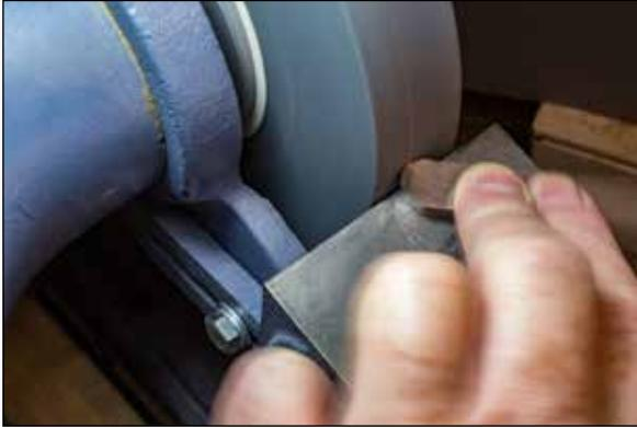
**Equalize** – Intentionally moving the sharpening position on the face of the wheel can equalize wear and minimize gulleys.
