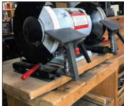
**Baseboard** — Rubber feet stabilize the baseboard under this transportable grinder.
