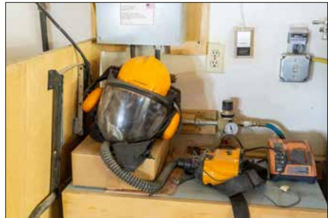
**Protection** – While somewhat cumbersome and pricey, a self-contained, powered filter helmet using a HEPA filter provides excellent breathing protection.
