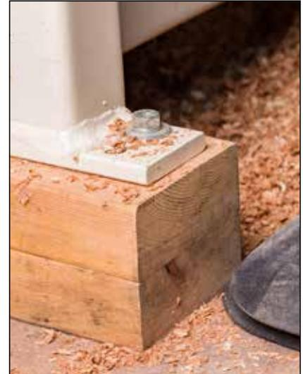
**Change height** – Blocks raise the lathe. Build a low platform to raise the turner. Be certain to include the mat thickness in your calculation.
