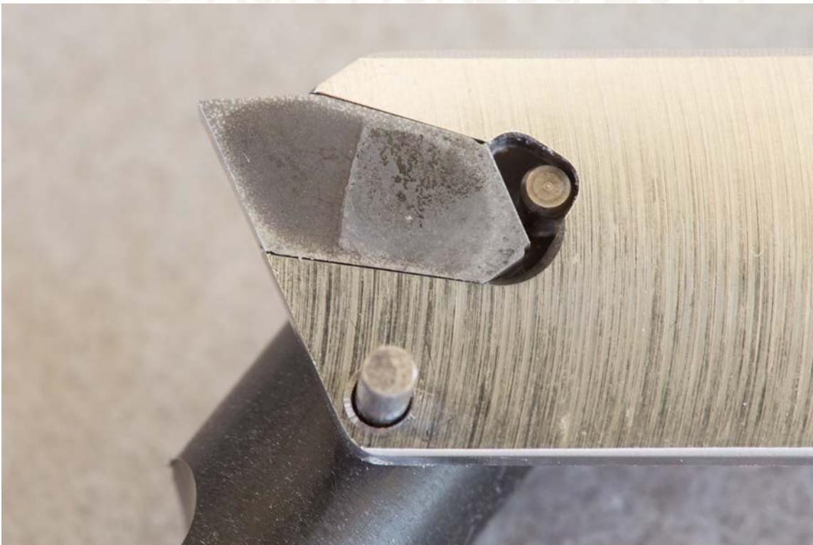
Figure #12: A view from the working side. The long rod in the hole under the cutter and the short rod located anywhere in the slot behind the cutter readies it for cutter release.
