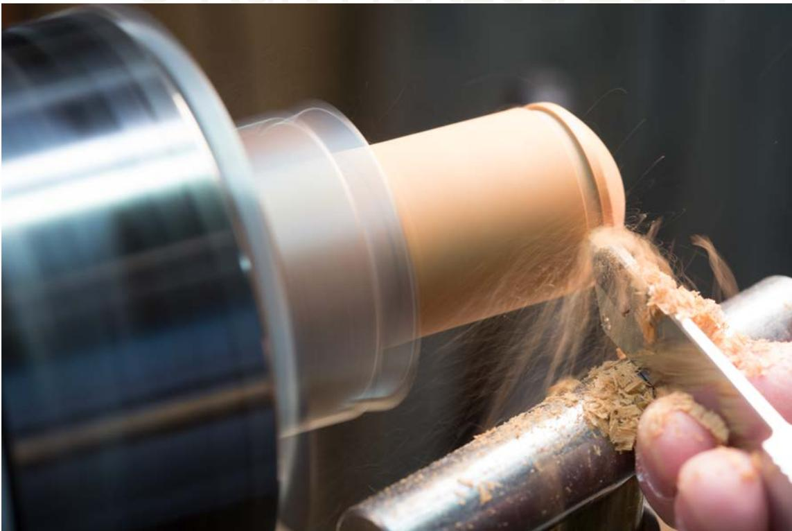
Figure #4: In use, it works exactly as the other parting tools you're used to. The full length handle is unique in the industry offering advantages in leverage and comfort with size of work.
