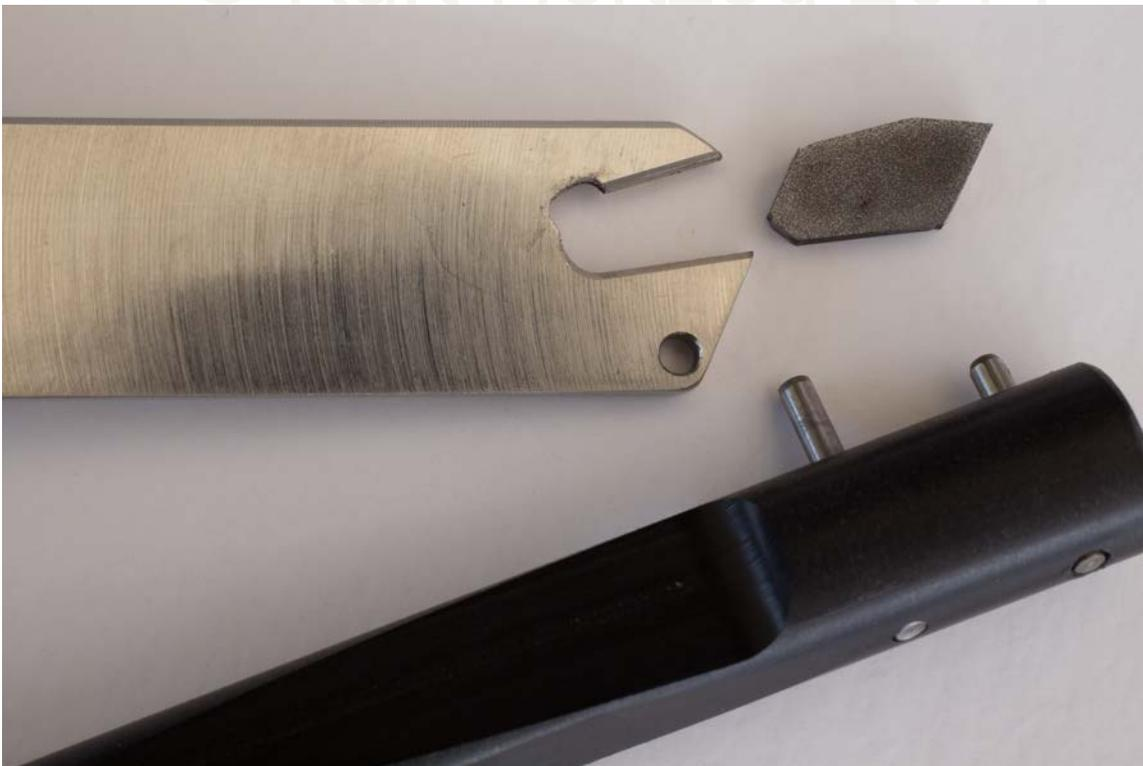
Figure #16: The unlocked carbide cutter is now removed by hand. It can now be swapped for a replacement cutter or touched up with a diamond hone if you desire.
