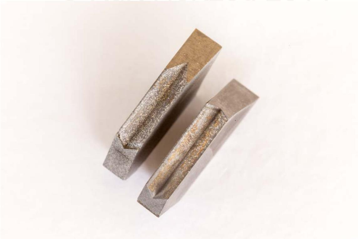
Figure #20: The trick to getting the carbide cutter to lock into place is the brilliant locking notch system in the tool. The carbide cutter has a V notch molded into the top and bottom.
