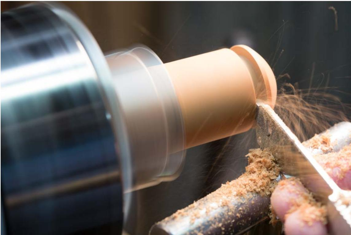
Figure #5: Even though the wider cutter face cuts a small clearance to minimize friction and heat generation, good practice is to “stair step” your cut.
