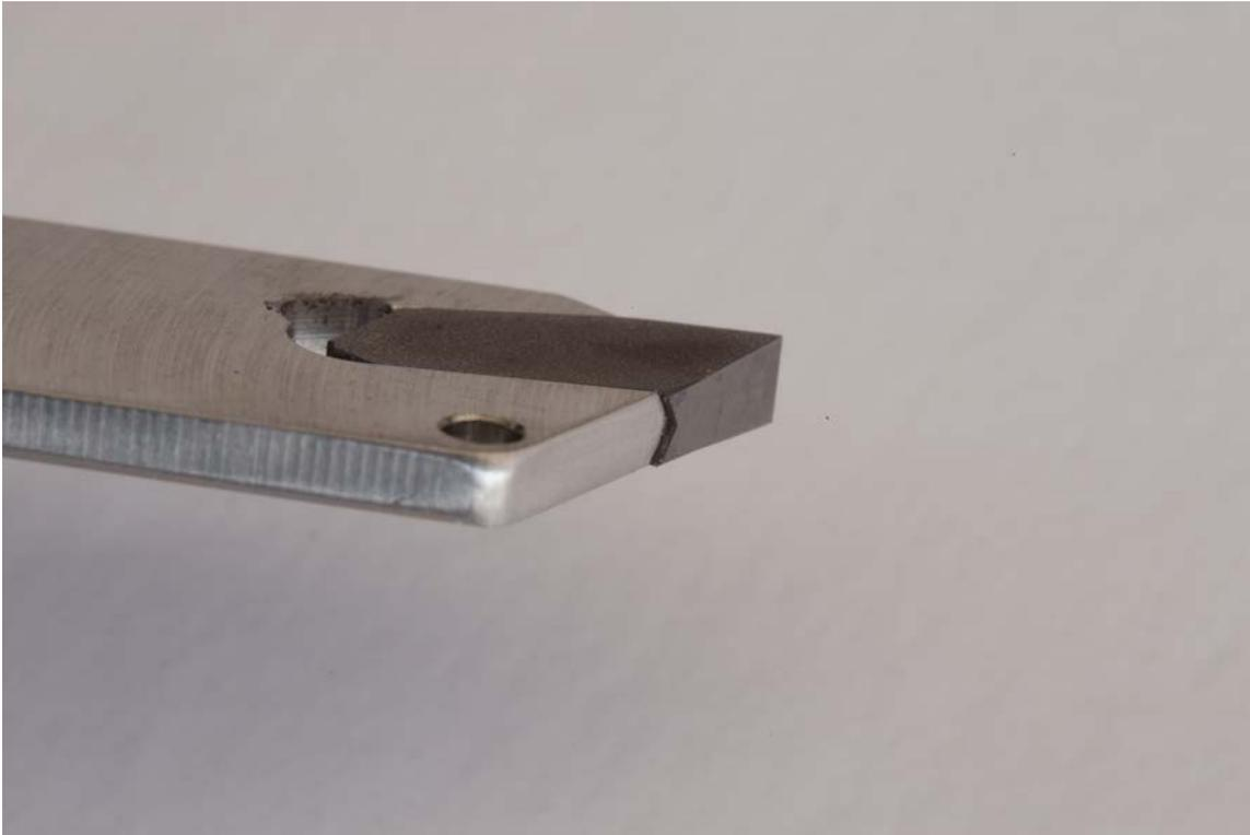
Figure #15: The amount of protrusion is indeed very small yet that is all that is needed to free the cutter from its seated ready for use position.
