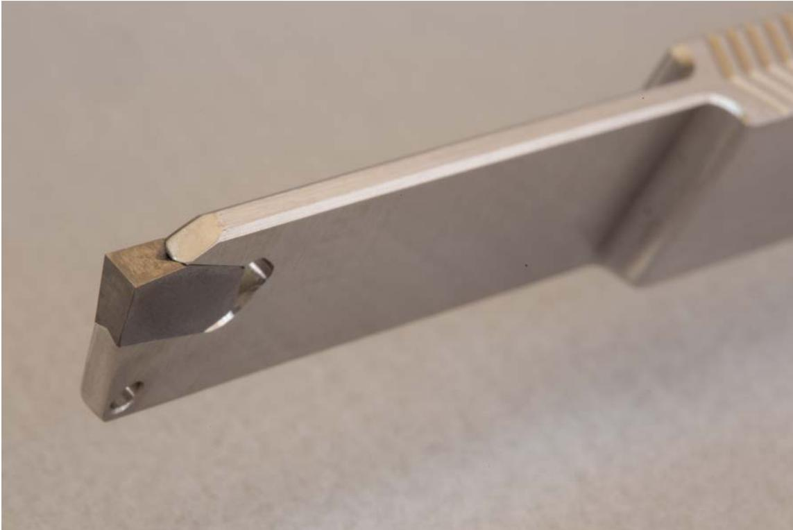
Figure #3: The business end of things is the 6" of tool extending from the 20" overall length with the 1/8" wide carbide cutter on the end.
