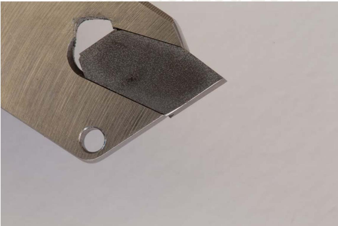
Figure #14: Shown loosened, the cutter extends only a small amount proud of the steel tool face. Being “unlocked” at that point, it is ready for changing.
