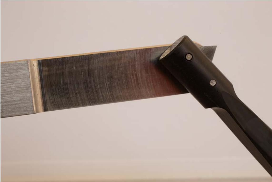
Figure #11: The shorter post is placed in the opening just behind the cutter. A very easy movement of the EWT Flex Key frees the carbide cutter allowing for replacement.
