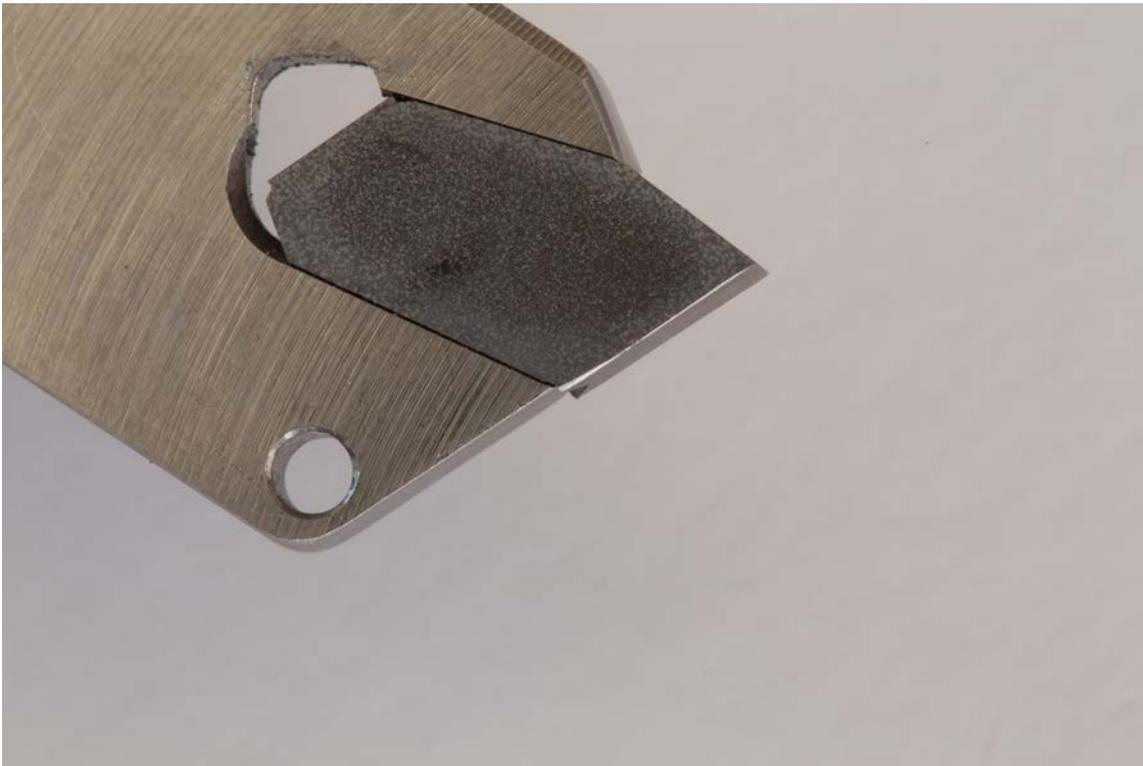
Figure #17: The replacement cutter is positioned in the tool as shown. No force is needed to get it to the proper position for seating with the EWT Flex Key as it easily slides into place.
