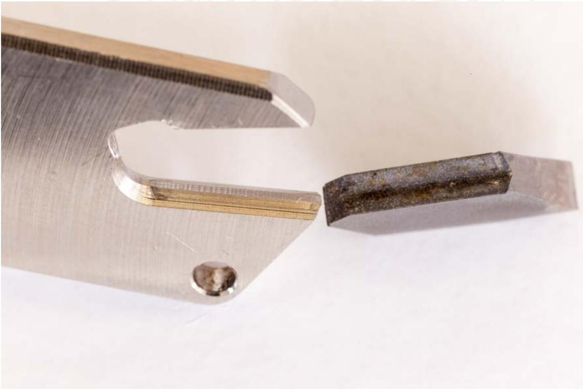
Figure #22: That same V mating face is machined into the bottom face of the cutter slot. These two V faces lock into the V slot features in the carbide tool locking things in place.
