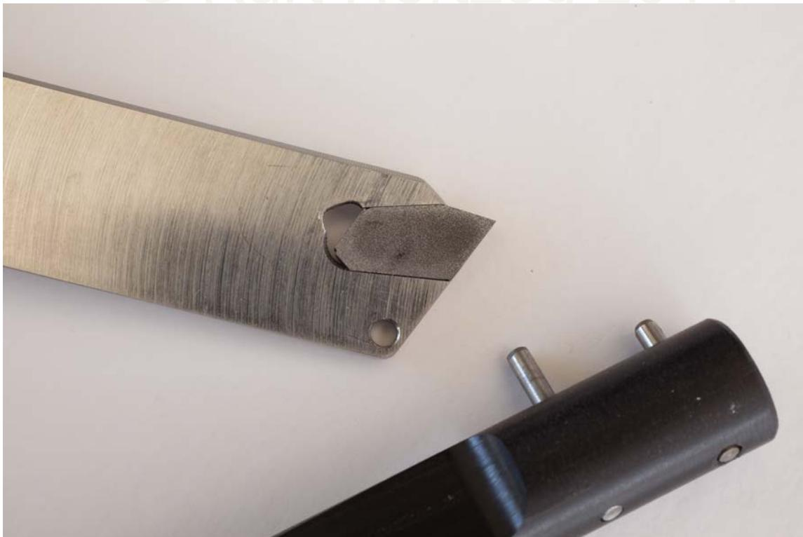
Figure #10: Its use shown very well in their instructions, the EWT Flex Key has one post longer than the other. The longer post is placed in the hole in the tool below the carbide cutter.
