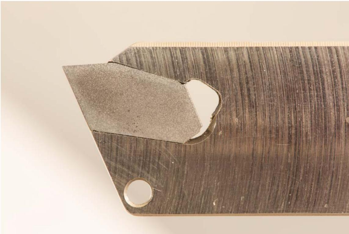
Figure #19: A small rotation of the EWT Flex Key around the long post in the hole on the tool seats the carbide cutter into the proper locked position indicated by flush on the front face.
