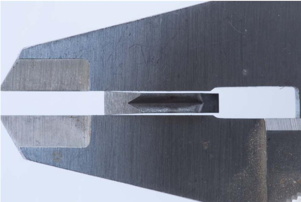
Figure #7: Cleverly designed to cut its own clearance, the front face of the cutter is 0.125" while it necks down to a shade over 0.100".
