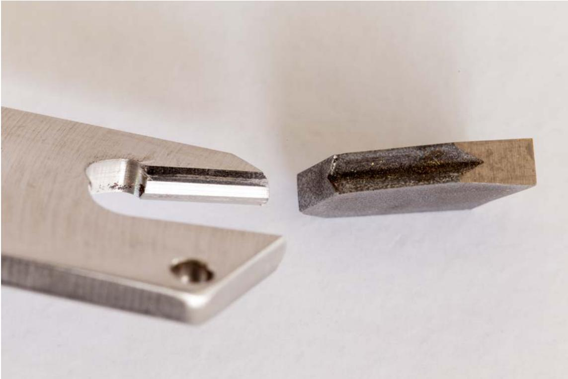
Figure #21: There is a mating V milled into the top of the tool that will lock into the V on the carbide cutter.
