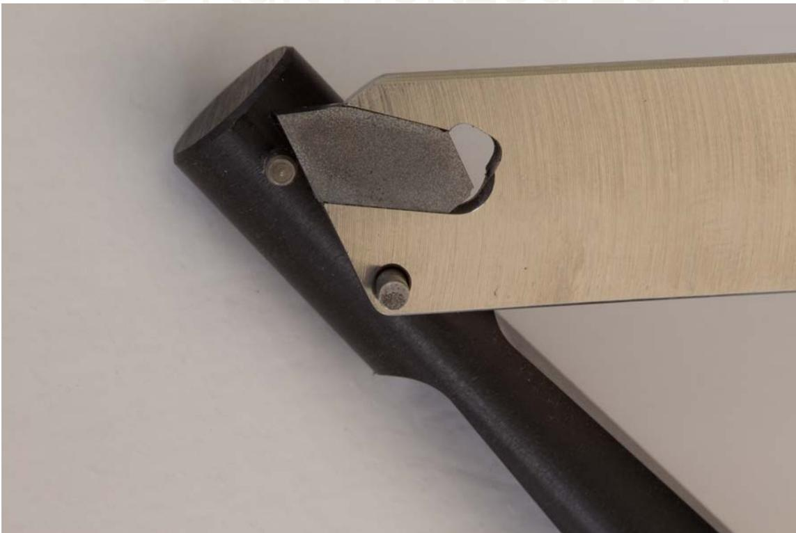
Figure #18: The seating process still uses the long post in the hole on the tool but now the short post is positioned on the front face of the carbide cutter.
