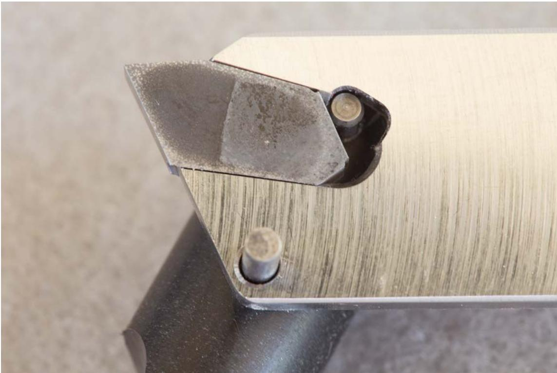
Figure #13: A slight rotation of the EWT Flex Key moves the cutter forward unlocking it for removal. The short rod will hit the stop position to prevent launching the cutter.
