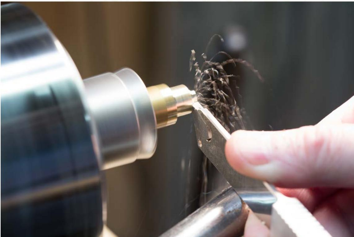
Figure #6: The full length handle allows for better control and the carbide cutter makes this parting tool ideal for materials in addition to wood. It works nicely on soft metals as well.
