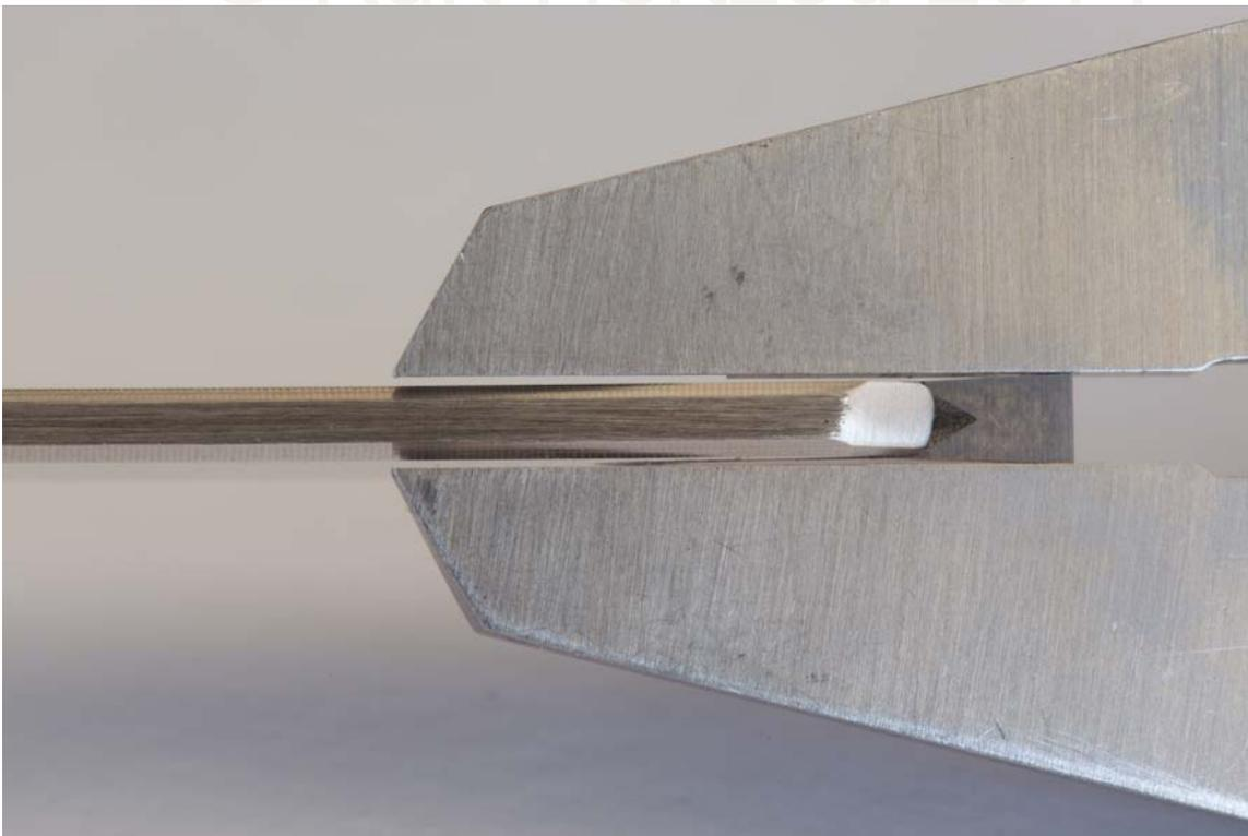
Figure #8: The tool mirrors this thinned tool thickness being just proud of 0.100". With the first 2 1/2" of the tool having of this thinned wall, it can fit into just about anywhere.
