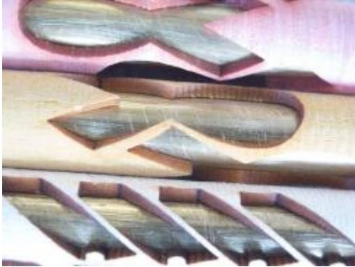
Figure 4 - The remainders are perfectly cut but have nonsensical patterns since the harvesting is for maximum material utilization.
