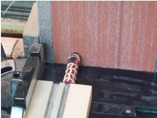
Figure 33 - The pen blank, piloting on the I.D. of the brass tube, can be sanded accurately and perpendicular to the brass tube.
