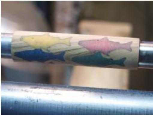
Figure 39 - Turning and sanding can proceed as usual. Any small voids or air holes can be filled with Ca.
