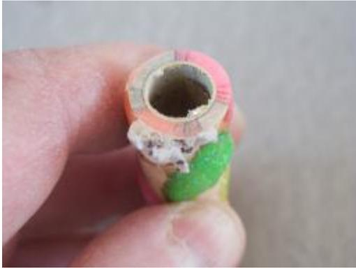
Figure 36- After length trimming, you can see how well your tube to wood bond and tube to filler bond turned out.
