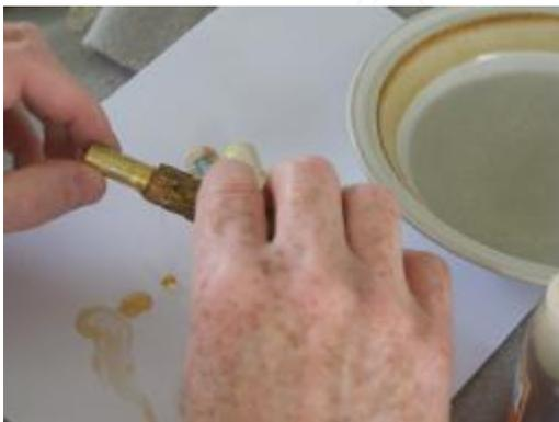
Figure 26 - I use polyurethane glues to bond in my brass tubes after scuffing the tube, spreading the glue on the tube, and wetting the inside of the blank with water.
