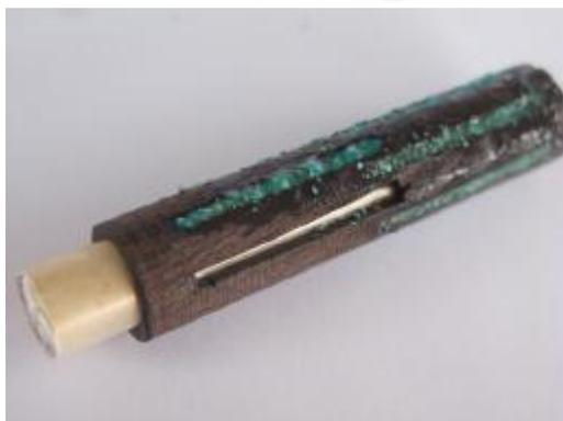
Figure 16 - Multiple openings can be filled, bonded, and then rotated to work on the next area making filling and material loss at a minimum.
