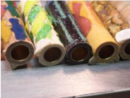
Figure 34 - Since the pen assembly sizes on the length dimension of the brass tube, it is important that the blank be trimmed only until the wood is just flush with the brass tube.
