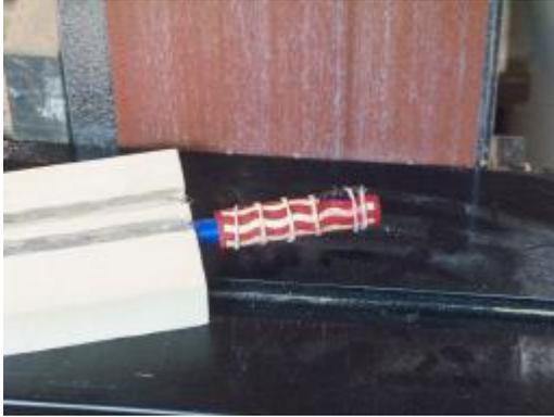
Figure 32 - My home built sanding jig allows me to sand the end of the blank flush to the tube on my belt sander in order to reduce stress on laser cut blanks, including remainders.
