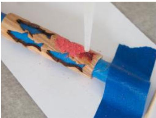
Figure 8 - One technique for solidifying the inlayed material is to drip cyanoacrylate glue into the opening to fuse it together.
