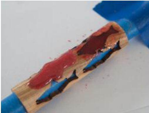
Figure 11 - The filled epoxy can be put into the opening with care taken to insure good perimeter wetting and adequate material to allow for any shrinkage.
