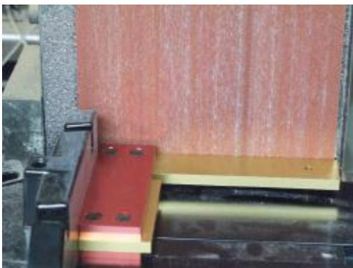
Figure 31 - The sander belt platen also needs to be square to the fence on the belt sander table.
