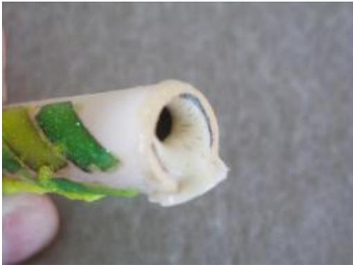
Figure 28 - I like to see a generous amount of adhesive that has foamed out each end indicating good coverage over throughout the brass to wood bonding area.
