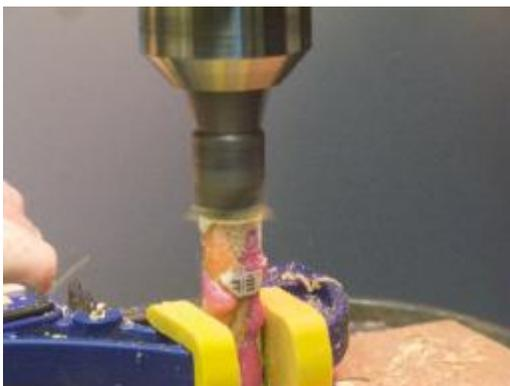
Figure 35 - The non-fragile pen blanks can be trimmed using the traditional rotating pen mill piloting on the I.D. and trimmed only until flush with the brass.
