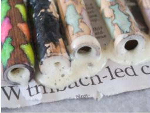
Figure 27 - The curing polyurethane will foam out the ends and often spread inside the tube but it is easily cleaned up after it has set.
