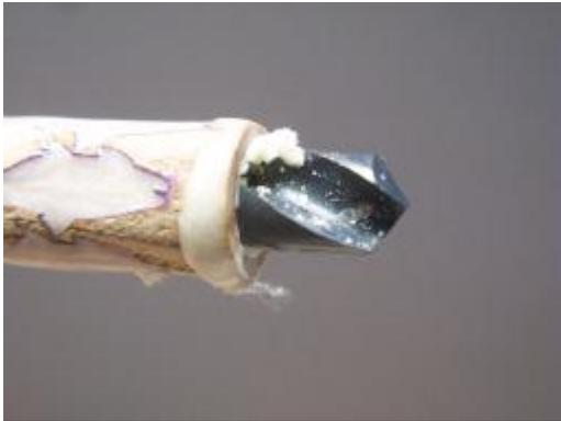
Figure 29 - The proper sized drill, used with hand power, will clean out any excess adhesive that has plugged the end or infiltrated the I.D. of the brass tube.
