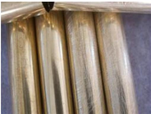
Figure 24 - I am a fan of scuffing the brass tube to help remove the drawing lube and oxidation from the tube prior to gluing it into the pen blank.
