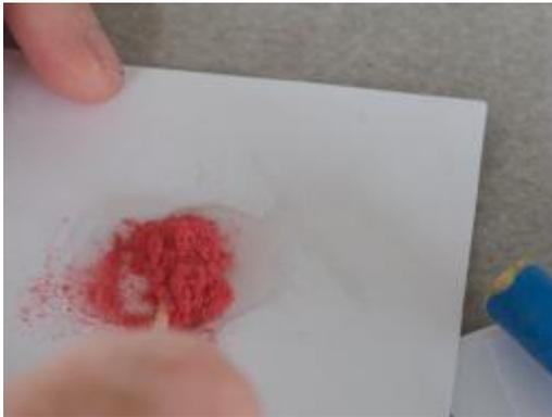
Figure 10 - The final color and ultimate density can be controlled by the quantity of filler used in the mixed epoxy.
