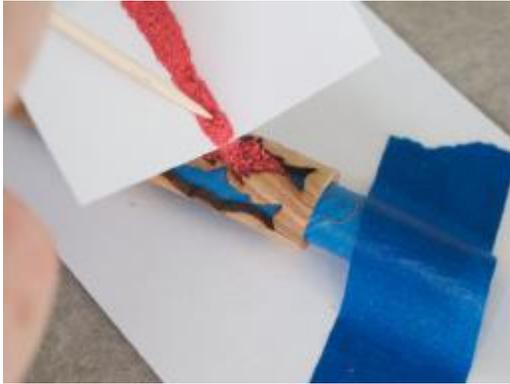
Figure 7 - By providing a backing in the cutout area, filler materials can be put into the opening to create a unique style pen blank.
