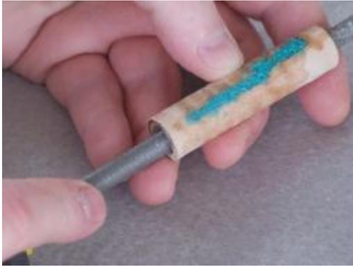
Figure 23 - It never hurts to rough up the inside of the blank to provide a good surface for the adhesive when fastening in the brass tube.
