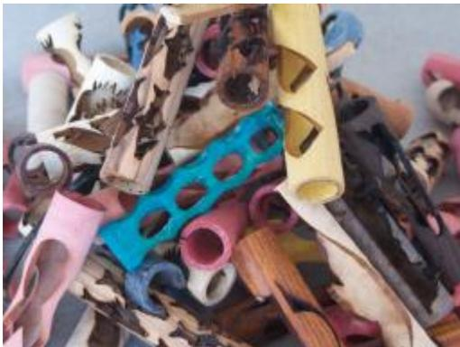
Figure 3 - The need for many different colors of wood creates a large number of scrap pieces after many inserts have been harvested from them.
