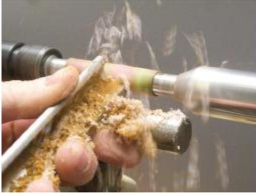
Figure 38 - The pen blank can now be turned using your preferred tools and method with any changes as needed based on your inlaid material
