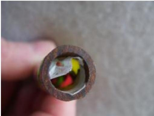
Figure 20 - On occasion, the waxed paper wrapped around the tube to prevent bonding to the tube gets stuck to the inside of the tube.
