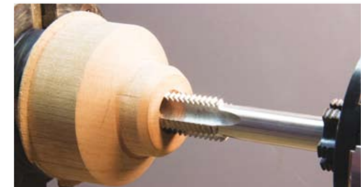
The keys to accuracy and repeatability are cutting mating flanges, perpendicular and parallel mating surfaces, drilling/tapping, and turning as needed with a single fixing on the lathe
