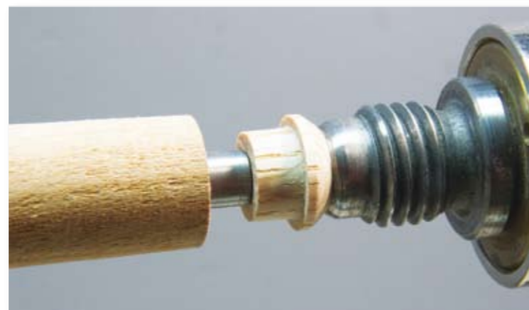
A mandrel saver doesn't get much simpler or less expensive than a scrap piece of oak turned to fit in the centre point hole, bearing on the lead in angle, with a 6mm hole bored for the mandrel shaft
