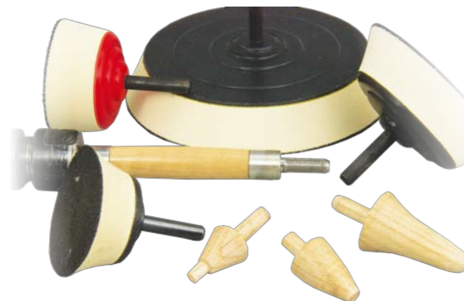
A bonus is that the mandrel shaft diameter is the same as many shaft mounted accessories making your mandrel saver a multi-purpose attachment system. Bought or made, 6mm shaft fits
