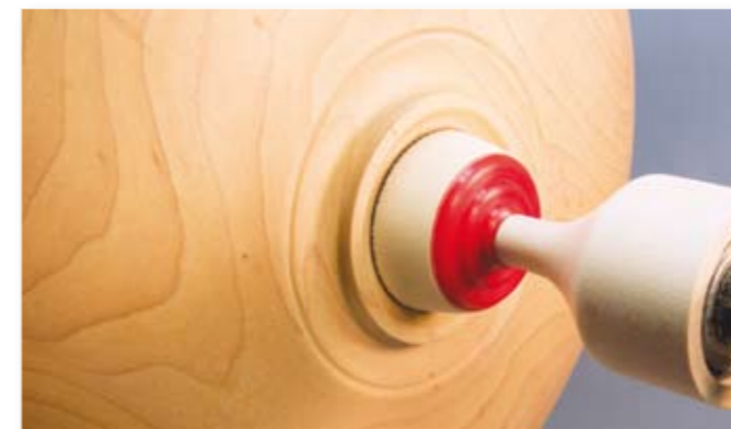
A sanding pad with no abrasive used as a padded tailstock fitting. There is no relative motion between any of the tailstock fittings presented. All make use of the tailstock centre bearing rotation
