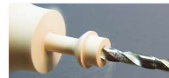
All of the processing done using a secure single mounting is one of the keys to accuracy and repeatability. Every remounting brings the opportunity to introduce error
