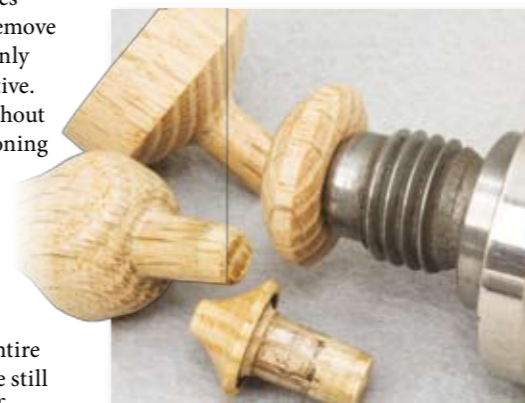
For quick yet durable fittings, oak works nicely. These fittings are pressed into the hole after the tailstock point is removed
