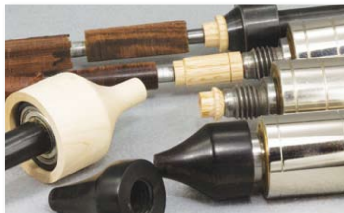
An assortment of homemade mandrel savers with mounting or attachment from the quick and dirty to the permanent including slip over, threaded, centre point/nose push and internal bushing
