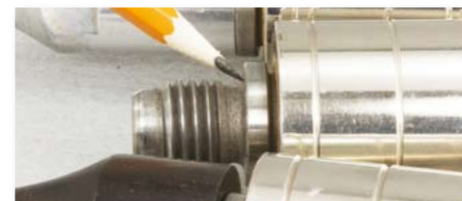
Thread to thread lockup provides no fastening accuracy. Accuracy and repeatability requires that the flange on the tailstock centre spindle be pulled to and held securely against its counterpart on the fitting
