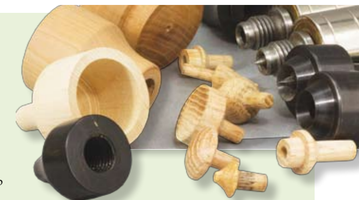
Whether inexpensive or expensive tailstock centres, here is a method to build a system of custom made tailstock fixtures. This system will allow you to buy or create your own workholding aids as needed
