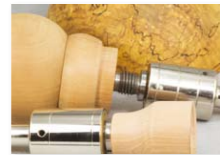
You can create a quick 'cut to fit' tailstock centre piece that can be used with the centre point and front flange. Long term use might involve better mounting methods such as threading
