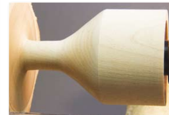
A slide over style of fitting is easily made by boring the proper sized hole with a Forstner bit then turning to need
