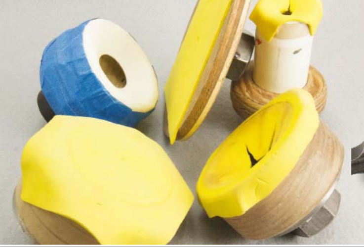
Easily made with low cost or scrap materials, these homebuilt workholders are multi-tasking. They can be friction drive or vacuum chucks and platens
