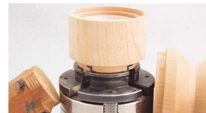
Marking your chosen jaw position (I use No.1), you can usually reposition your homebuilt chuck mounted workholding drives accurately by 'feeling' the indents as you position and tighten
