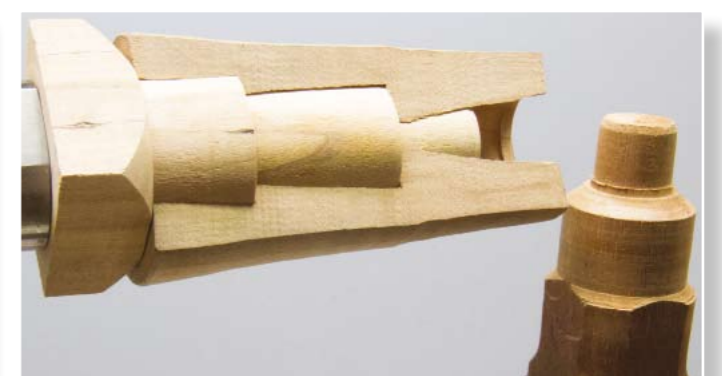
Don't forget threading your creations for accuracy and repeatability. Facing, tapping, then turning your drive on that mount will allow will work nicely. Here, peppermill mandrels
