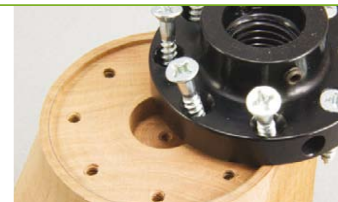
While changing faceplates in and out isn't recommended, it can be done. Giving the faceplate an accurate surface and positional lock will allow for good re-installation accuracy
