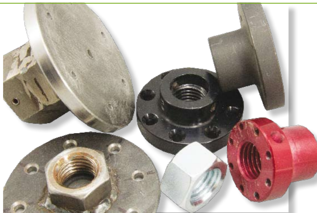
Your homebuilt jam chucks, pressure plates, vacuum chucks, mandrels and more become very accurate and repeatable using faceplate mounting. An embedded nut also can work nicely
