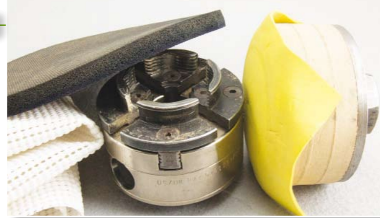
Don't forget that your chuck with some padding becomes as effective as the purpose made friction drive. While the chuck can't double as a vacuum chuck, it certainly is readily available
