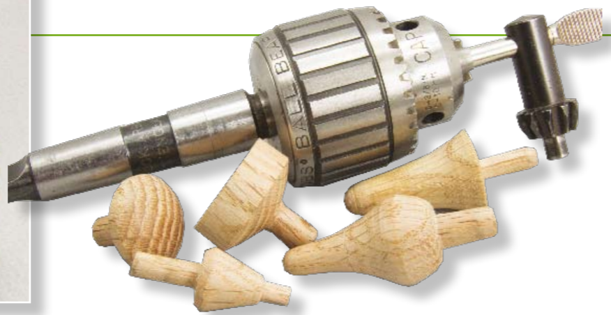
Creating small form fitting drives for those special needs it easily and low cost. Your Morse taper drill chuck is the ideal universal holder for these
