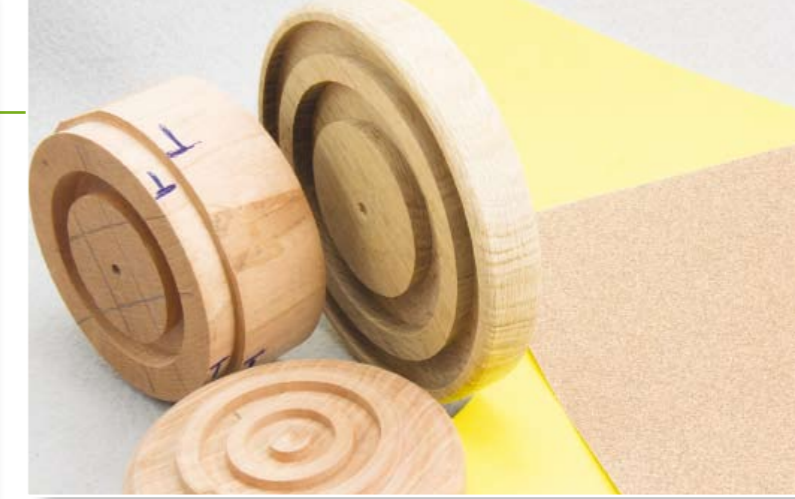
The two chuck grip sizes on the multi-point jam chucks work with #2 or #3 jaws. The oak platen has the same and can be a pressure pad or lathe mounted sanding/sharpening plate depending on your choice
