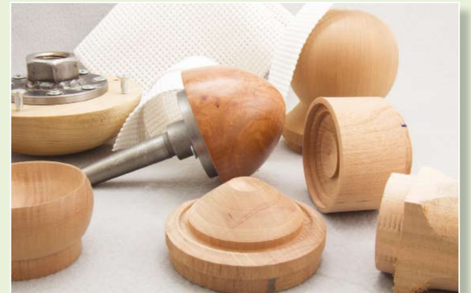
Headstock creations allow you to make those custom drives that help solve your workholding problems. Low cost, easily made, and tuned to fit, take advantage of the creative possibilities
