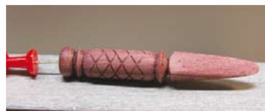
The last usable piece turned into a letter opener albeit not a very large one. The push pin in the back was used to help hold and orientate the letter opener as it was presented to the belt sander for blade sharpening
