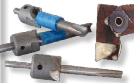
Painter's tape also makes a useful barrel trimmer pilot size adaptor. Wrap the tape around the shaft to take up the space needed and avoid the chatter of the cutter when facing the end of a pen blank. The tape is easily applied and removed as necessary, and is certainly convenient
