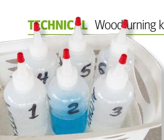
For using chemicals, I favour pouring some from the large storage containers into properly marked dispensing containers. Not only are the quantities in the work area much smaller, but the dispensing is more measurable and therefore accurate. Safe handling always!
