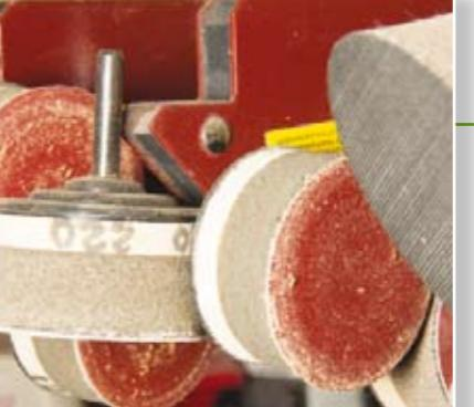
Sanding pads are of low-enough cost to dedicate a pad to each abrasive. Marking them clearly helps you insert them in the drill, use, clean if needed, and return to the magnet quickly. You can have a set for each durometer pad you regularly use
