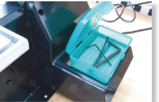
For tools and equipment needing adjustment, keep the required sizes of Allen keys, wrenches and other items in a dedicated storage container. A soap container fastened with double-sided tape keeps the three Allen keys I need with my mini bandsaw
