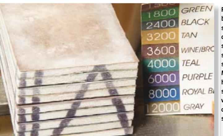
Remembering some bizarre colour-coding scheme or trying to determine an abrasive sequence with shopworn fingertips seems silly. A simple Magic Marker-triangle helps me sort the sequence visually and very quickly. I use the other marks to help me speed orientation
