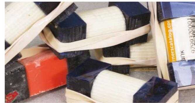
A bag of rubber bands will find plenty of use in the workshop. I use rubber bands extensively as glue clamps. The compression is controllable and squeeze-out is of no concern since I cut right through them as scrap when turning
