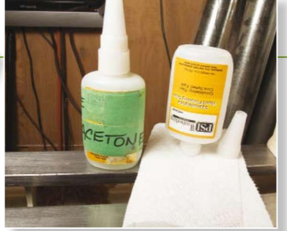
When using CA adhesive, I recommend having a small container of acetone or other debonder open and within reach. Far too often a spill will attach you to things that make it difficult to reach the debonder, much less open it!
