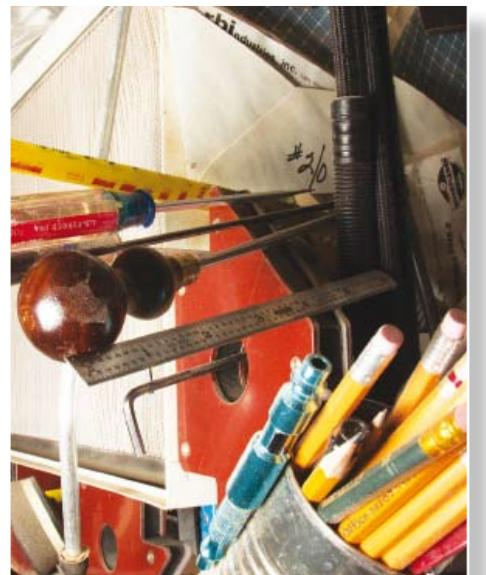
I use welder's magnets in the workshop to fasten items I need at their point of use. Metal rules, scratch awls, cut-off saw blades, tailcentre knockout bars, tins of sharpened pencils, etc. are all located at my lathe. I have different items stored at the bandsaw and drill press
