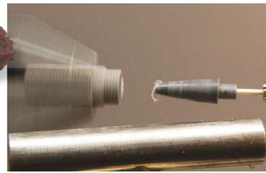
A toothpick or bamboo skewer works wonderfully to keep small objects from disappearing into the chips when parting off. You can then focus on the parting process rather than catching the turning as it is freed from the lathe
