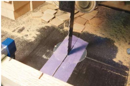
Low-tack painter's tape works well for everything from masking turnings for sprayed finishes to closing the size of your bandsaw's throat plate. Keep rolls of the tape at different locations throughout the workshop so that it is always to hand to solve any immediate problems
