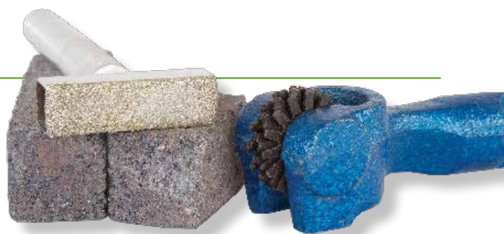
Wheel dressers from old to new. The 'devil stick' – lower left – is from another time – with the star wheels – right – not far behind. The most modern and effective diamond dresser is in the upper left
