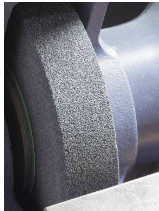
A properly dressed wheel will be flat across the face with the colour being 'dull'. The absence of shiny spots, embedded steel and the dullness indicates fresh sharp cutting particles ready to work
