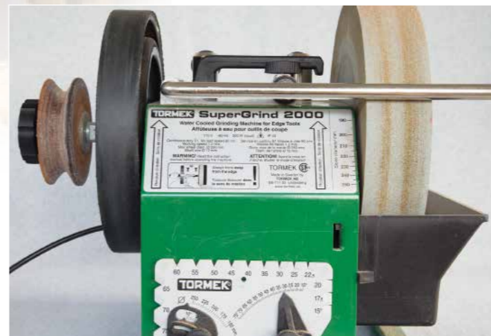
The Tormek or other water wheel sharpening systems offer a larger wheel diameter and a finer grit size. There are jigs and fixtures available to accommodate woodturning tools
