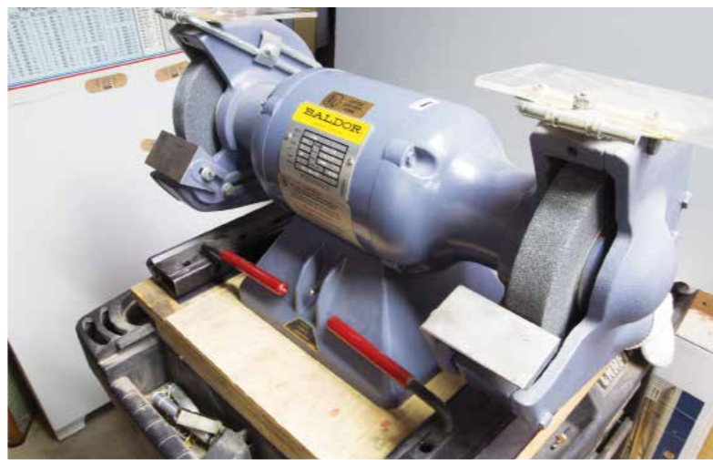
Regardless of the rests that are installed on the grinder, a sharpening system benefits from having an after-market grinding fixture system. This accommodates those special needs effectively
