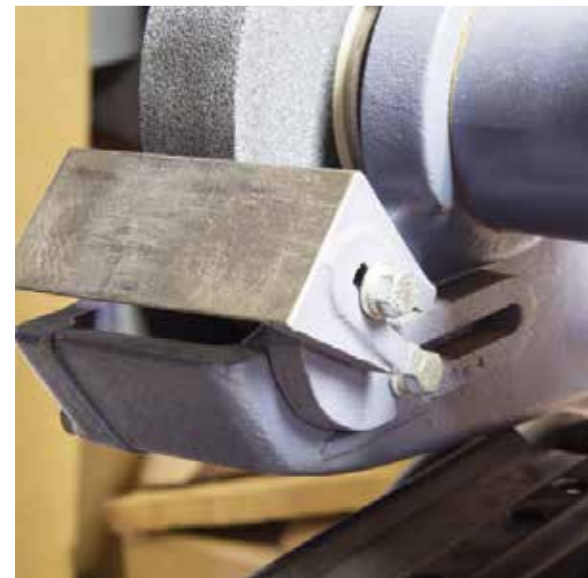
Regardless of the rests that are installed on the grinder, a sharpening system benefits from having an after-market grinding fixture system. This accommodates those special needs effectively
