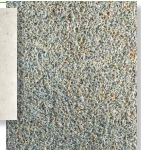
Wheels coloured white are usually an indication of high friability or the ability to break down during use to present unused and sharp particles. Wheel dressing will accomplish the same function, and on demand
