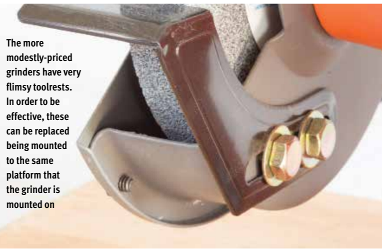
The 200mm bench grinder offers the advantages of a gentler-radius hollow grind and the ability to house 25mm wide grinding wheels. Available in both high and low speed as desired
