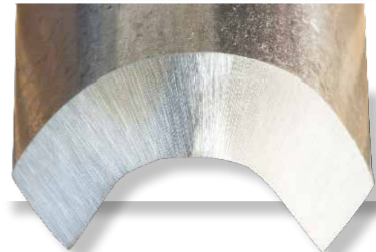
Grit selection is a balance of steel removal capability and fineness of ground edge. A look at the end of the tool will tell what grit grinding wheel was used
