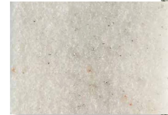
Wheels coloured white are usually an indication of high friability or the ability to break down during use to present unused and sharp particles. Wheel dressing will accomplish the same function, and on demand
