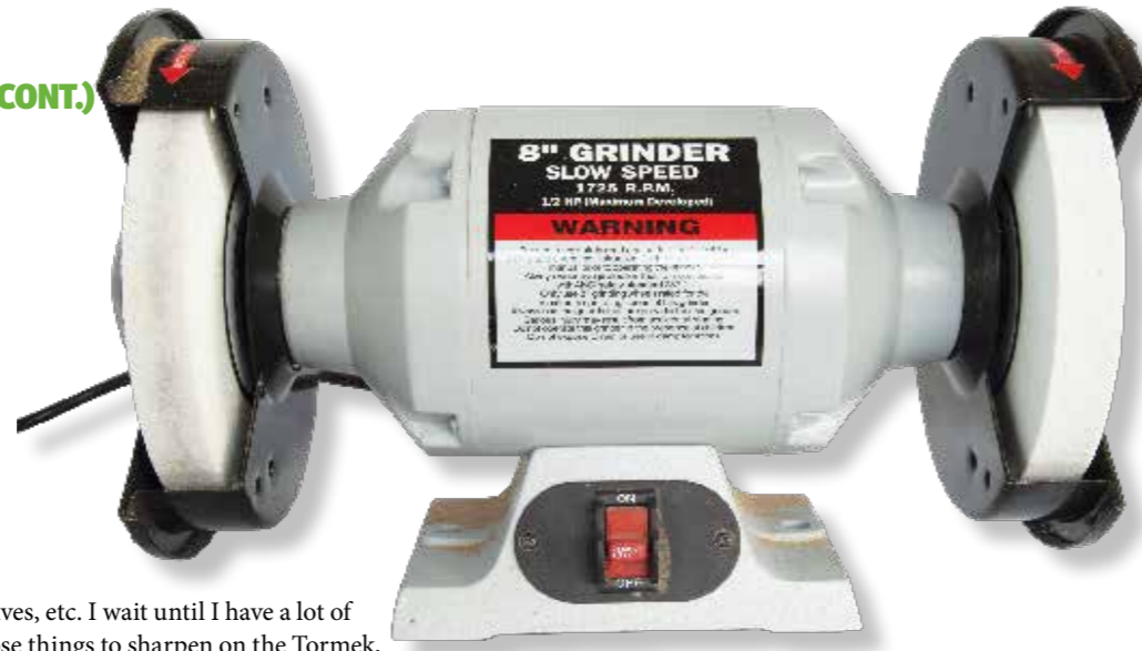
The 200mm bench grinder offers the advantages of a gentler-radius hollow grind and the ability to house 25mm wide grinding wheels. Available in both high and low speed as desired
