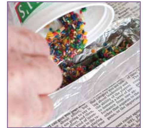
Mixing your filler to completely wet the surface will help create a good blank. Longer open time materials help let any trapped air escape to the surface
