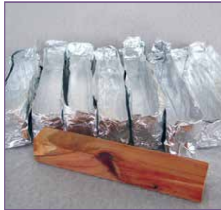
Regardless of the size or purpose, foil moulds using a pattern can be made. Folding heavy duty foil to avoid any seams will create a serviceable mould
