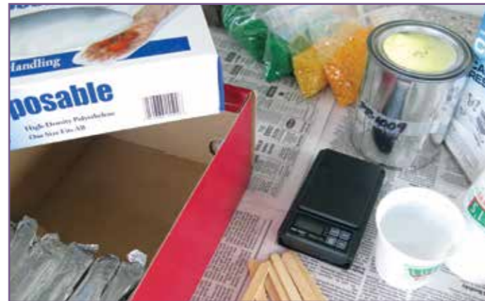
Having your work area layed out including table coverings, moulds, resin and catalyst, PPE and scale will help prevent scurrying and unnecessary spilling
