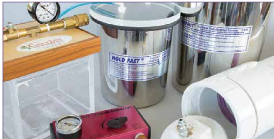
Rather than using pressure to minimise entrapped air, I'd rather use vacuum to draw the bubbles to the surface. Your chamber and vacuum source will work
