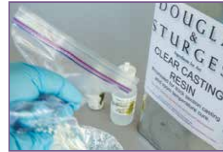
Better than removing entrained air bubbles, don't introduce them. A polyethylene bag will let you mix the two by kneading and then pipette it out
