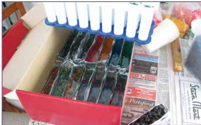
If there are long side walls needing support, stacking moulds side by side in a shoe box or placing blocks to prevent flexing will work
