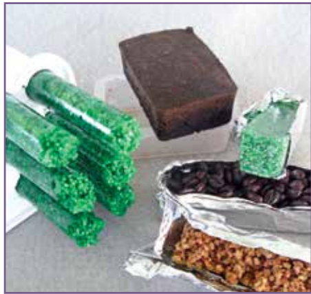
Of all of the moulds I've used, I find my own homemade moulds with aluminium foil are the most flexible, lowest cost and easiest to use
