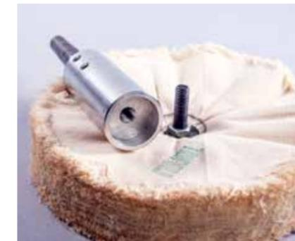
I favour the version that mounts in my lathe. The adaptor fits into the taper and provides the proper threading to receive the various buffs
