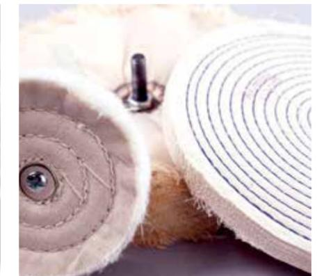
Buffers are available in different materials, diameters and rigidities. By stitching the buff, the pattern and nearness to edge controls the stiffness
