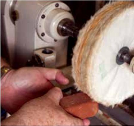
Charging and recharging the wheel with buffing compound is a simple task. Done below centre with an easy touch, the wheel is lightly loaded for use
