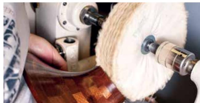
The key to good buffing is to use a mild pressure and let the compound do the work. When buffing, always keep the work moving to avoid burn through
