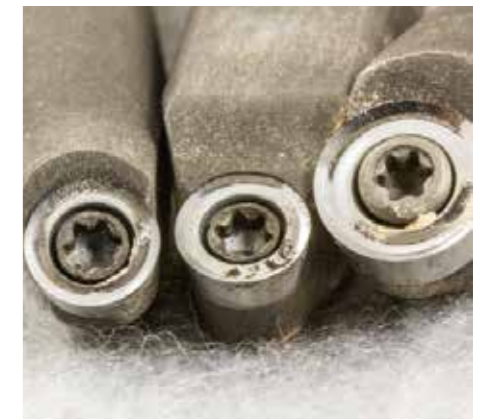
Most modern carbide cutter tools support the cutter as completely as possible. The cutter is exposed only in the areas of potential use
