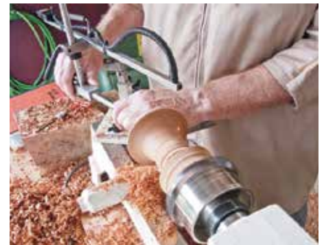
Adjusted for desired wall thickness, once the laser beam falls off the turning that dimension has been achieved
