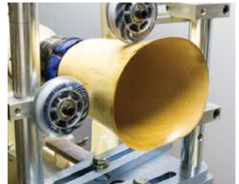
Turning a deep hollowing to a wall thickness of 1mm is achievable with use of a steady rest, a laser and care in turning
