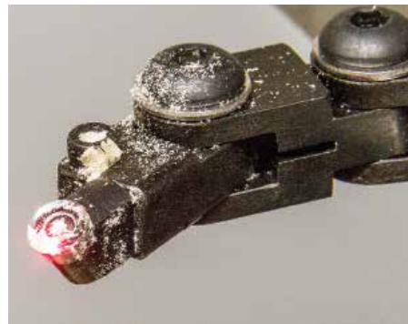
Depending on preference, you can adjust the laser to show cutting tool edge or set for a dimension away from the edge
