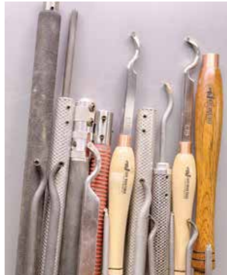
Both tool and tool handle length and mass have a dramatic impact on the length over the rest you can work safely. Select both carefully
