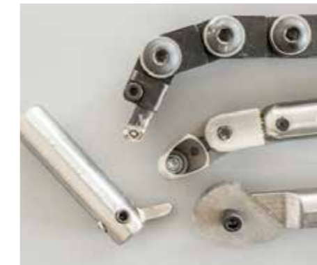
The mainstays of the hollowing tools for both the hand-held and the hollowing bar systems
