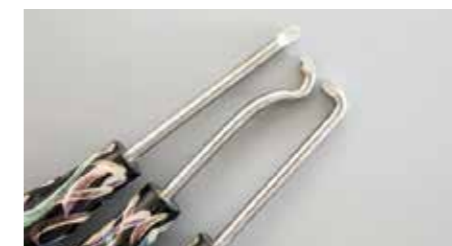
Originally, hollowing tools were just bent steel or tool steel usually bought unhandled. My early Chris Stott hollowing tools circa 2001
