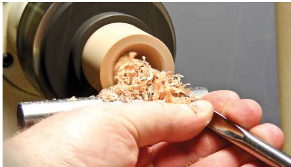
Drilling to set depth and hollowing can be done with standard gouges. Use the method you find safest and most reliable
