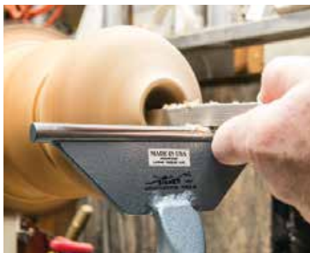
Safe hollowing demands support up close with sufficient toolrest strength along with tool shaft and handle appropriately sized
