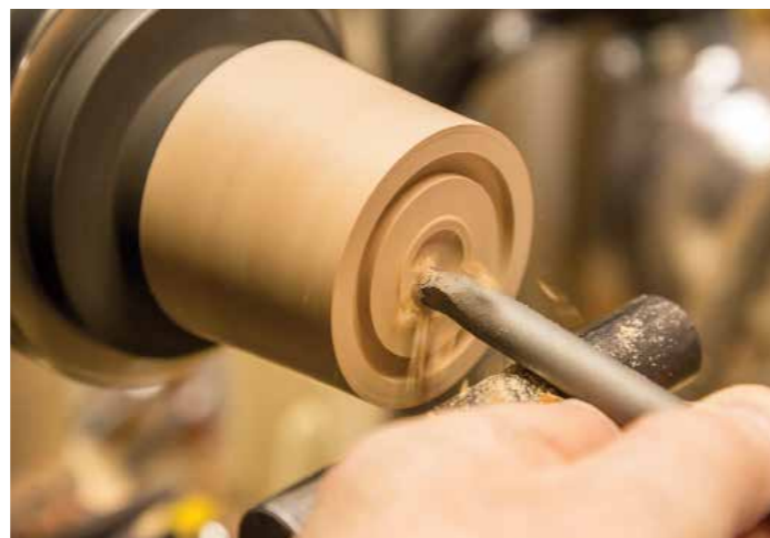
Hollowing lidded boxes is great practice. Notice the desired finished wall surface to work towards
