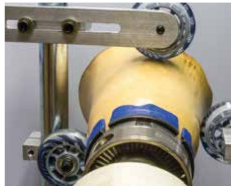
Using a quality, properly adjusted steady rest to minimise vibration and flexing maximises a laser's value on a hollowing system
