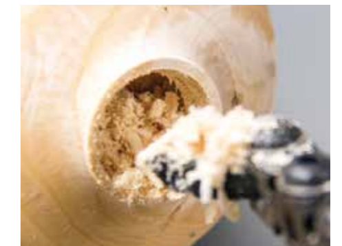
Regardless of your cutting sequence, the debris needs to be cleared from the turning to allow the cutter to effectively reach the surface
