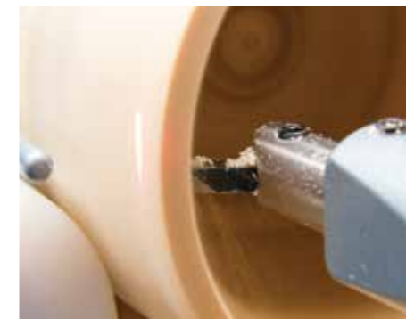
Cut to your finished wall allowing the material underneath to support your cuts working in shallow depth incremental steps. Step and repeat
