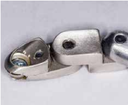
A shrouded/shielded cutter's aggressiveness is controlled by how much of the cutter is exposed from beneath the hood
