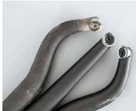
Carbide cutting tools are now available designed and manufactured for turning in forward and reverse. Remember to lock the grub screws
