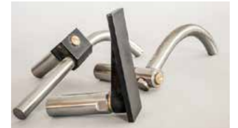
Speciality toolrests for support up close. Adjustable for reach or a platform for boxes. Beware of excessive demands placed on toolrests
