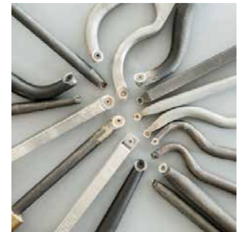
Just a few of the available carbide cutter hollowing tools for hand held use. All feature replaceable cutters when the existing has been rotated until spent
