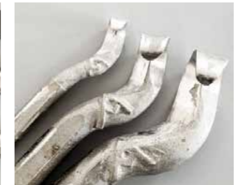
Superb at hollowing end grain green wood, the Martel hook tools are not for newcomers
