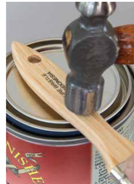
Sealing a paint can well will provide years of shelf life. Never hit it directly with a hammer. A piece of wood will prevent damage to the lid
