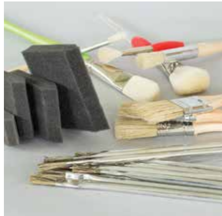
Milk paint can be applied with almost anything. The cheapest acid or chip brush to the finest artist brush will work. Properly thinned, it can be sprayed
