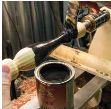
Milk paint loves bare wood. Once dried into the pores, it becomes nearly impossible to remove. Your lathe is a great workholding tool
