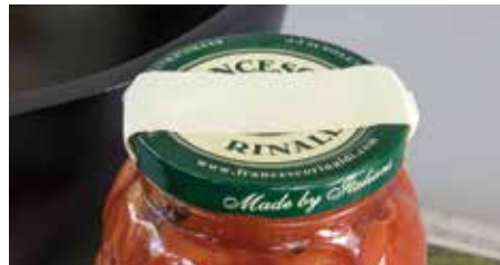
Need a spacer and holder to do the outside of a bowl? Some double-sided sticky tape on the lid of the right sized jar will work nicely
