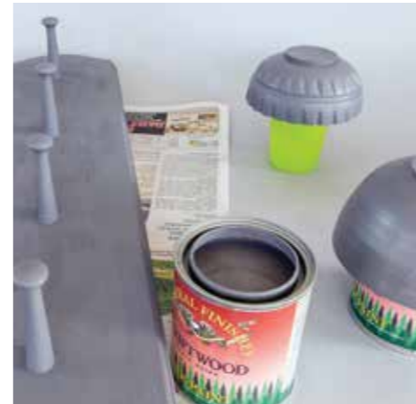
Milk paint often requires more than one coat. Plan on it and just apply generous even coats without touching up
