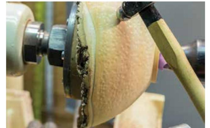
A simple ball peen hammer can be used to create that 'hand hammered' texture like metalwork
