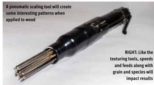
A pneumatic scaling tool will create some interesting patterns when applied to wood
