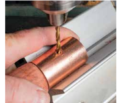
Drilling and tapping a ferrule is not difficult. Be certain you have or make a V block to assist
