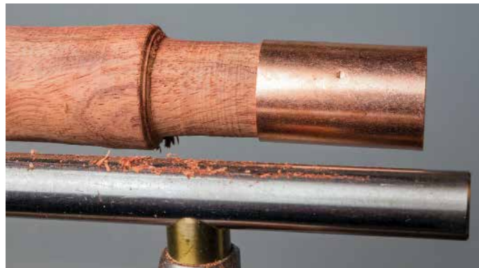
Rather than measure, I use the ferrule to test fit for size. Fast, easy and accurate. Turn until you like the fit
