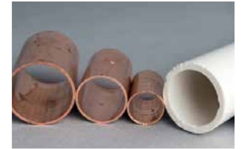
I've experimented with PVC piping for ferrules in low demand applications. It colours nicely
