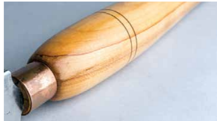
My favourite finish is Ca adhesive. After 15 years of use, this homemade tool and handle still look good
