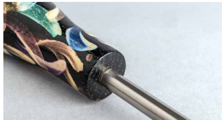
The easiest ferrule is no ferrule. My Chris Stott hollowing tools are light enough duty to require none
