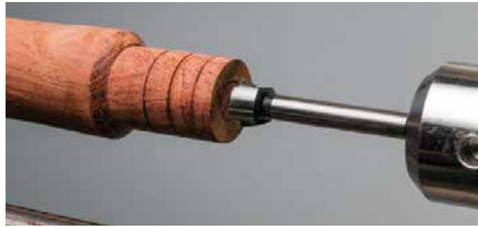
You can drill with a twist drill or a Forstner bit. The Forstner will give you a square bottom. Notice the cut in glue traps
