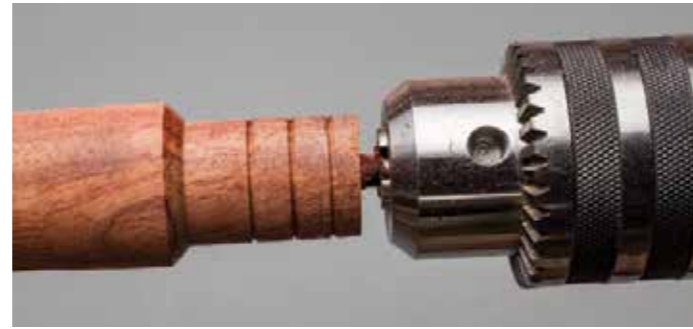
I know exactly my drill depth by setting the bit extension in the chuck and drilling to the chuck face
