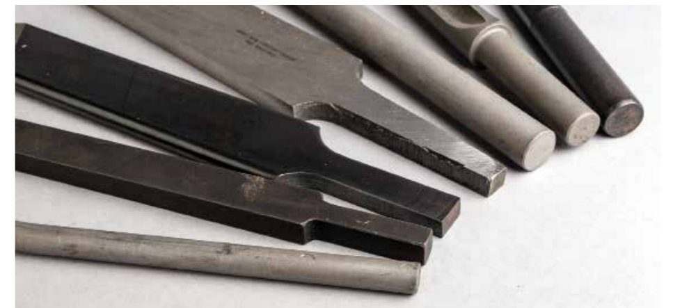
ABOVE: Your drilled size will usually fall into a couple of standard diameters but the square, rectangular and tapered vary. RIGHT: Adapters are available so you can accommodate a couple of different shaft sizes with one hole diameter
