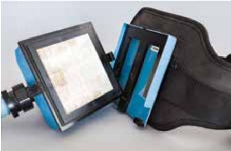
My older 3M powered filter helmet filters the incoming air through a HEPA filter which is on the belt behind me
