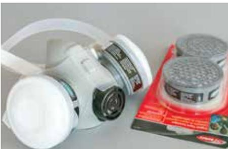
My vapour mask with the proper replacement filters. Keep extra filters on hand to allow changing when needed
