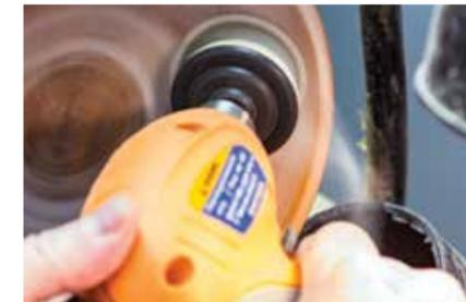
Locating an input to your dust extraction at the point of dust generation works well helping keep the air clean
