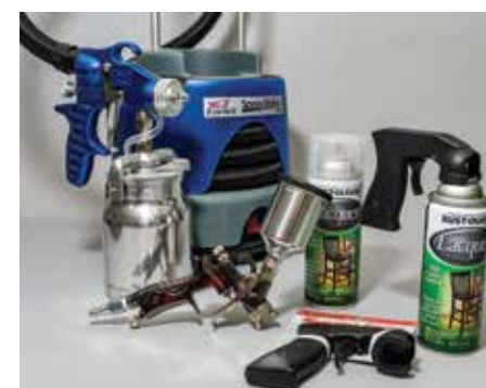
HVLP, standard spray gun, or rattle can aerosol dispenser. All work well but the aerosol requires no cleanup
