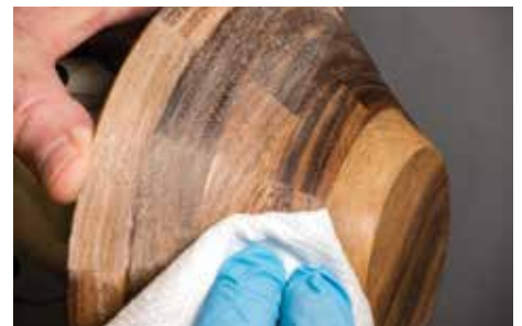
A good cleaning is needed to prevent embedding the debris in the next coat. I use denatured alcohol
